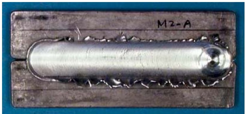
Figure 1-4 A Friction Stir Butt Weld Made of Magnesium Alloy (Li et al. [35])
