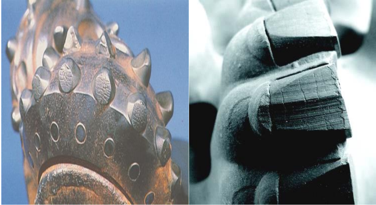
Figure 4: Bits overheating problem (www.smithbits.com)
