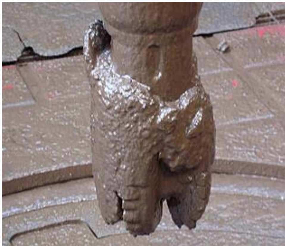
Figure 2: Bit balling problem (Drilling Formulas.Com)
