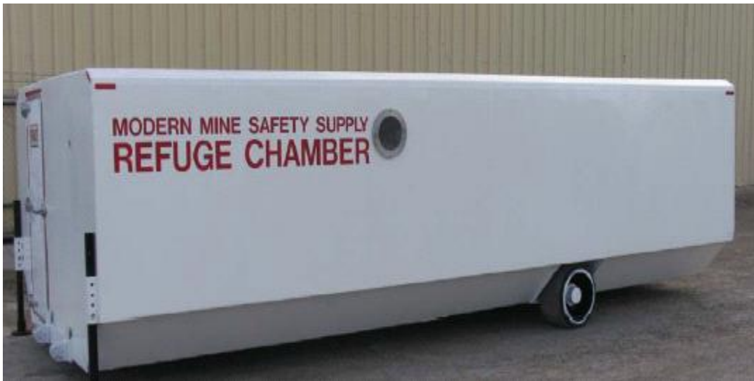
Figure 2-3. The Hard-Walled Shelter built by Modern Mine Safety Supply (MSHA, 2006)
