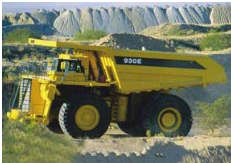
Figure 2-12. Komatsu 930E Heavy Diesel Truck with Electric Drive (Komatsu)
