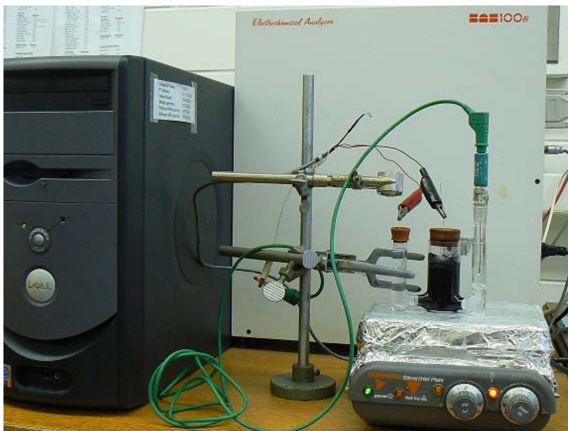
Figure 3-3. Electrochemical setup along with potentiostat
