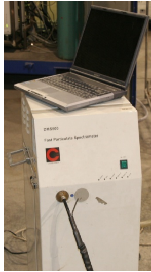
Figure 3-2: Cambustion DMS500 Fast Particle Spectrometer (cambustion.co.uk).
