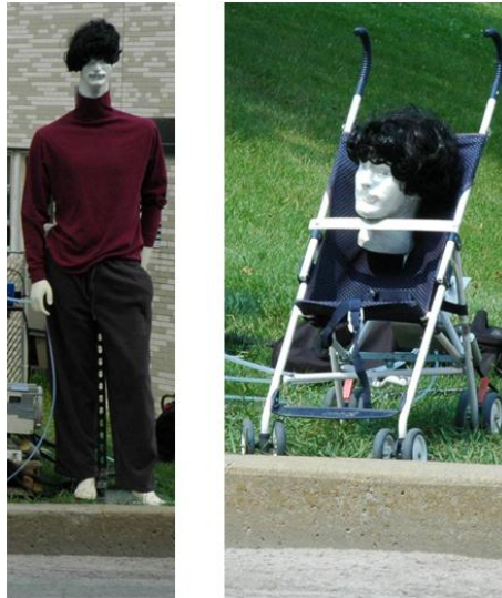
Figure 3-5: Pedestrian surrogate mannequin (left) mannequin's head simulation in stroller (right).
