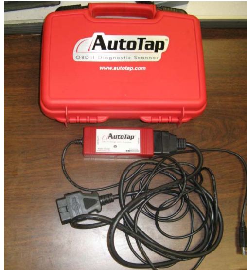
Figure 3-4: AutoTap OBDII Diagnostic Scanner.
