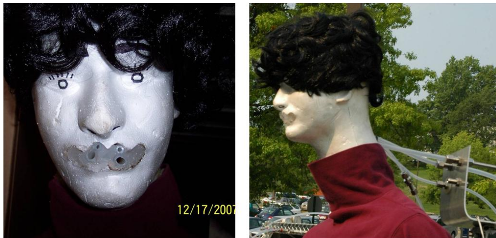
Figure 3-6: Mannequin's head with sample probes in mouth and attachment to sample tubing.
