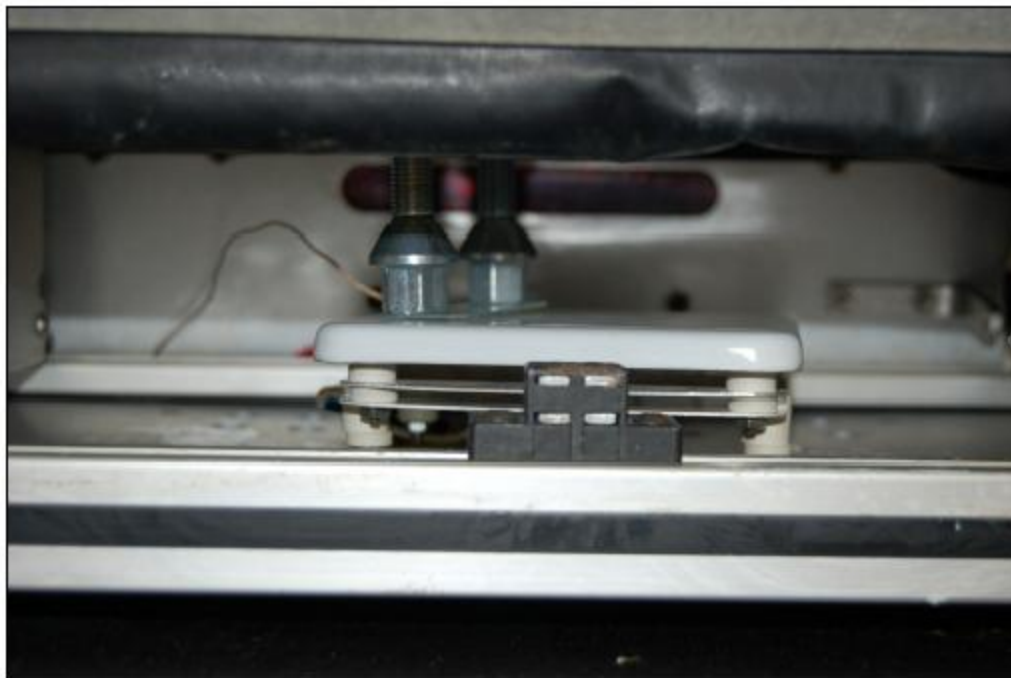
Figure 4.3-1: Thermocouple monitoring temperature of hot plate with weighted glass slide on top
