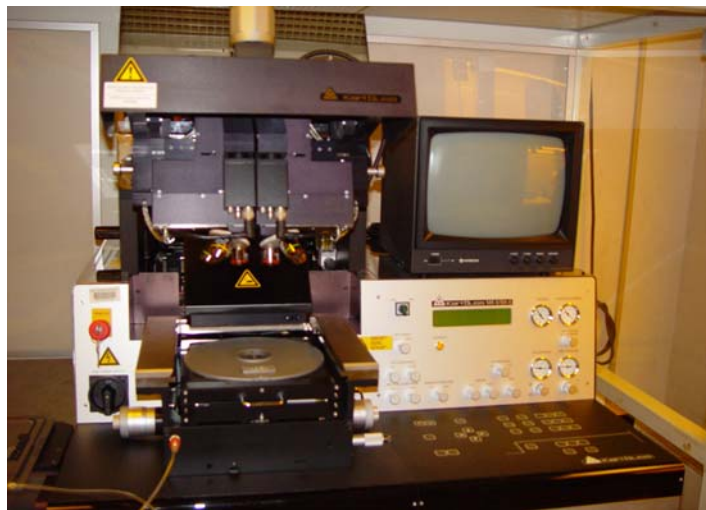
Figure 4.1: KarlSuss MA6/BA6 Aligner (Property of West Virginia University Micro/ Nanosystem Fabrication Laboratory)
