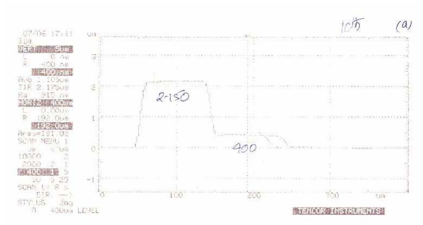
Figure 4.4: Alpha step profile of a step like structure
