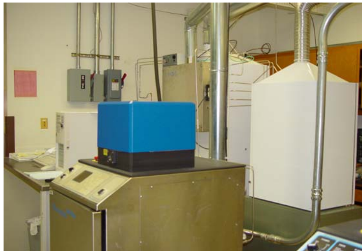
Figure 4.2: Oxford Plasmalab 80 plus PECVD system (Property of West Virginia University Micro/ Nanosystem Fabrication Laboratory)
