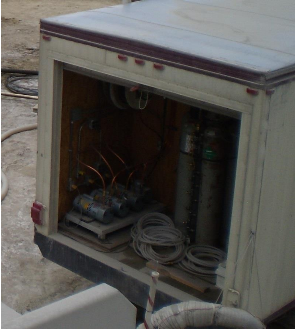
Figure 3-3. TBS trailer showing three large purge pumps (front), smaller sample pump (back), calibration cylinders for analyzer.
