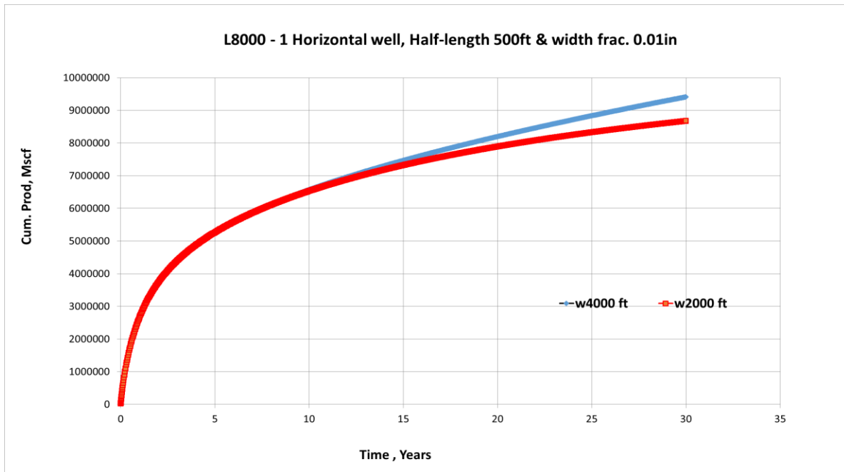
Figure A.9: Cumulative Production results vs. Time of hydraulically fractured horizontal lateral(s) – Results of Run 25 and 26 in Table 3
