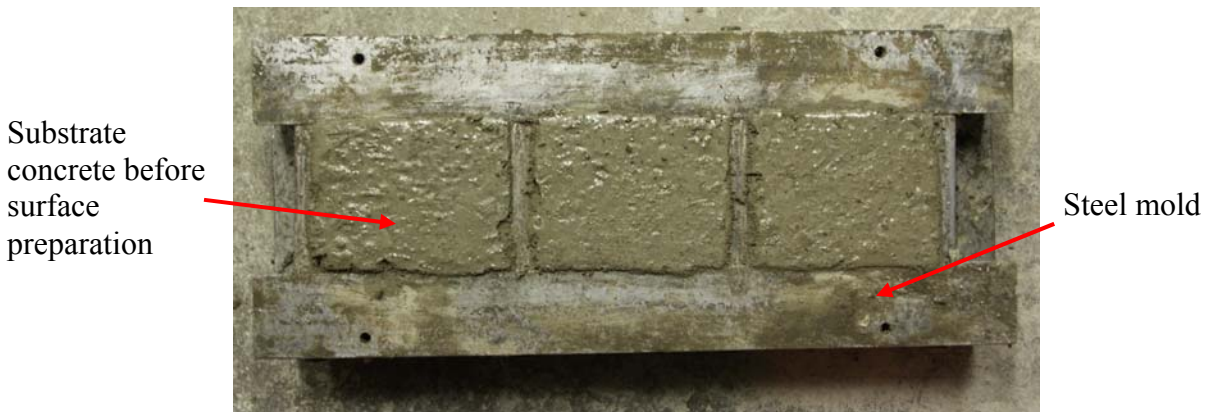
Fig. 3.8 Substrate specimens after casting
