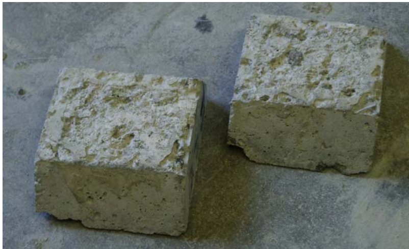
Fig. 3.10 Demolded substrate specimens
