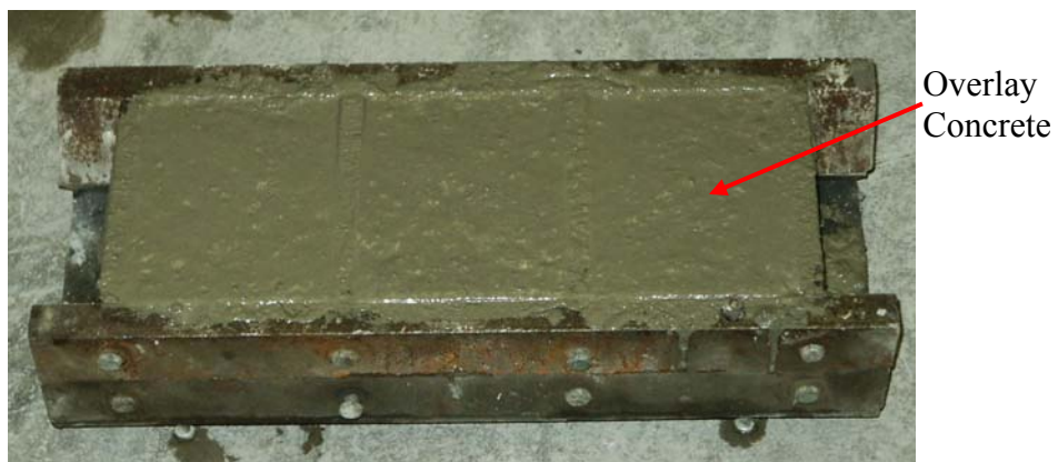
Fig. 3.12 Specimen after casting of overlay concrete
