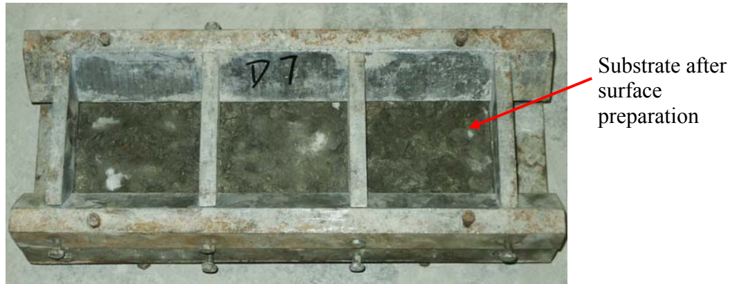
Fig. 3.11 Substrate specimens reinstalled back into molds
