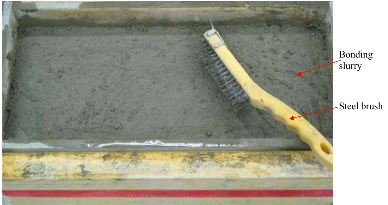
Fig. 3.5 Substrate beam with bonding slurry applied
