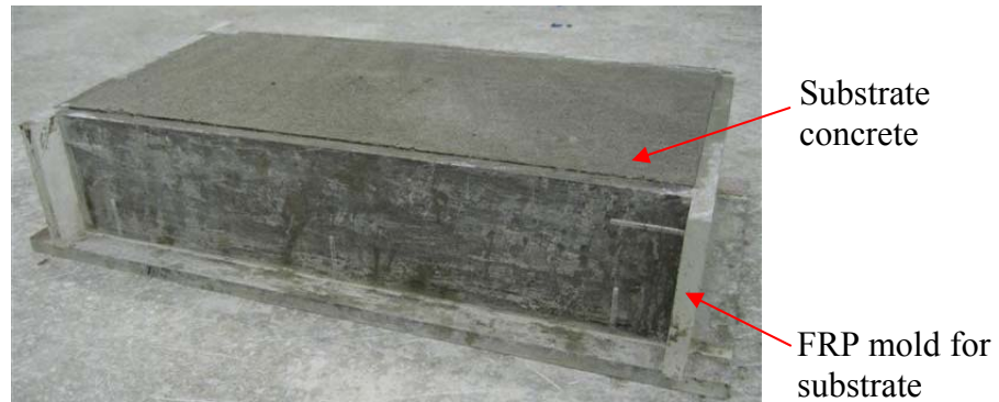
Fig. 3.1 Substrate specimen after casing
