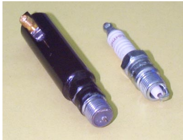
Figure 1 – The plasma igniter (left) and a conventional spark plug (right).
