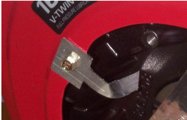
Figure 13 - The rigid pointer used to determine top dead center of the engine.
