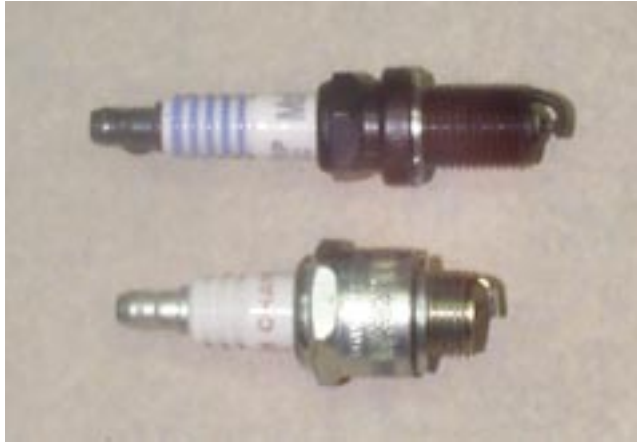
Figure 26 - The Champion model RC12YC (top) and model J19LM (bottom) that were used for initial testing.
