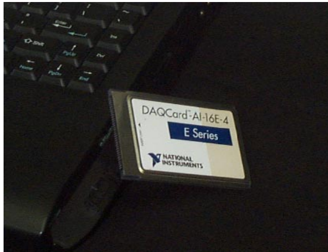
Figure 16 - The National Instruments model DAQcard-AI-16E-4 data acquisition card.
