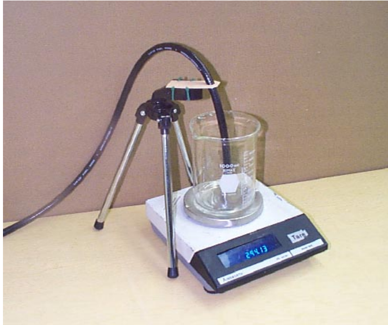
Figure 15 - The fuel flow measuring system.
