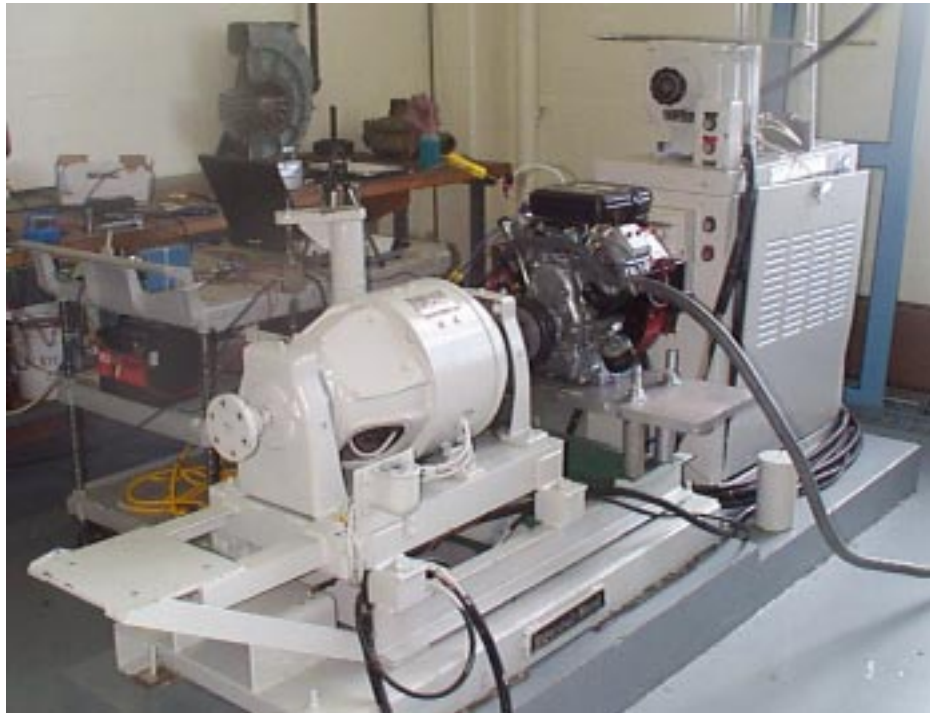
Figure 23 - The test engine coupled to the General Electric DC Cradled Dynamometer.
