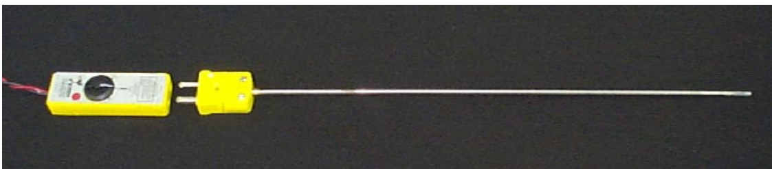
Figure 14 - The Omega model KQSS-18E-12 thermocouple and Omega model MCJ-K ice point device.
