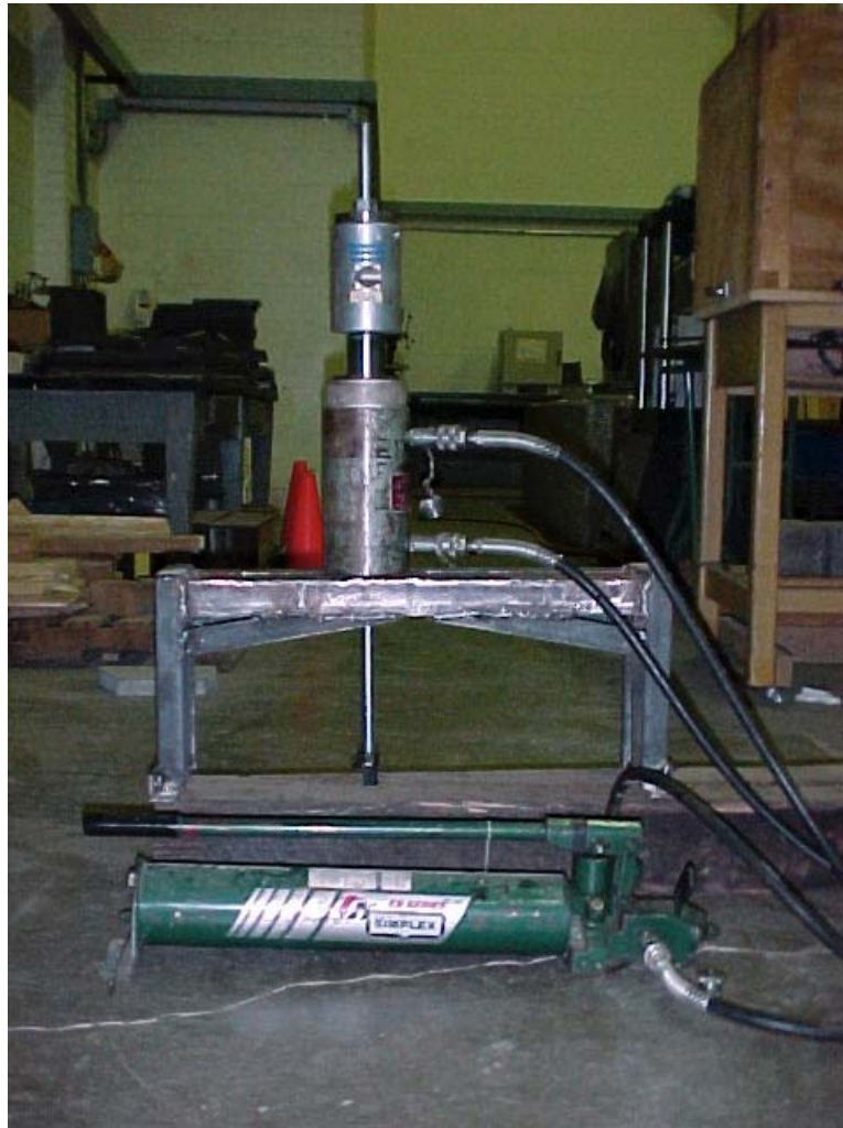
Figure 6.8 Set up of Pulling Spike Force
