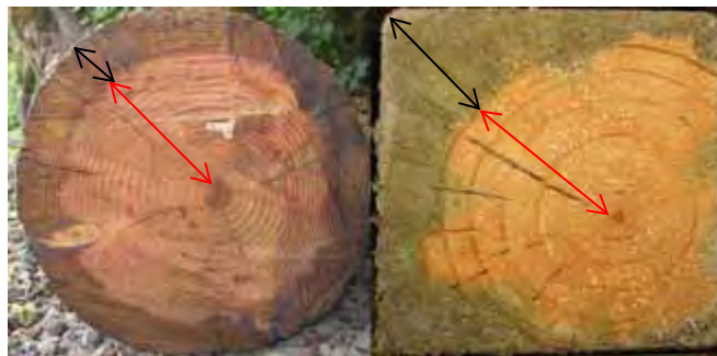
Figure 19 - Cross Section of Pressure Treated Wood Logs (Wood Handbook, 2010)
