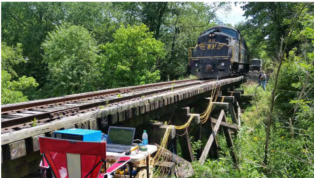
Figure 57 - WM 82 Locomotive Testing on Bridge 1.9 After Dump Truck Testing
