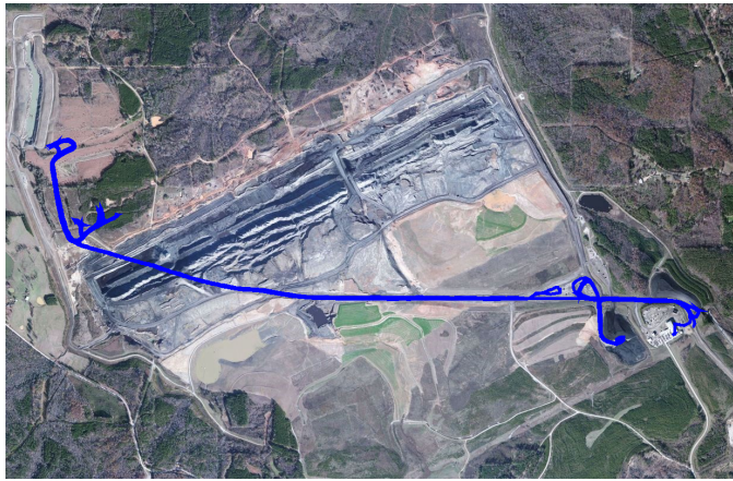
Figure 3.4: Sample track collected from the MapMyTruck for one of the trucks in Red Hills Mine on a working day
