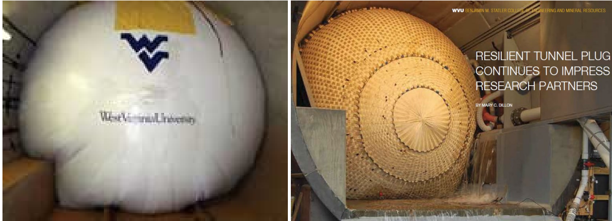
Figure 1.14: Plugs tested in an actual tunnel in 2008 (left) [14-15, 28], and in testing facilities at WVU in 2012 (right) [29].
