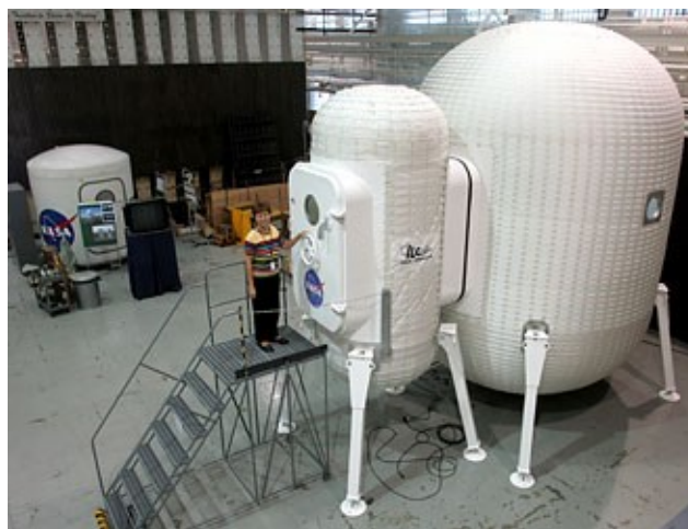
Figure 1.5: Aeronautic application: Inflatable Lunar Habitats [11].
