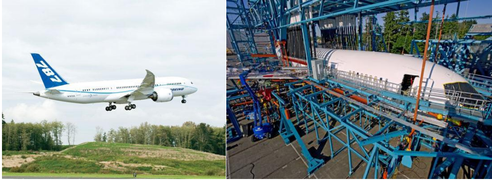
Figure 2.5 35 tons CFRP of fuselage, wings, tail, doors, and interior in each 787
