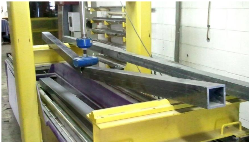
Figure 5.7 Example of FRP structural shape in 3-point bending (WVU-CFC)
