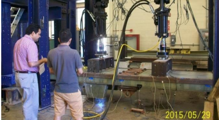
Figure 9.8 Four-point bending test on FRP wicket gate
