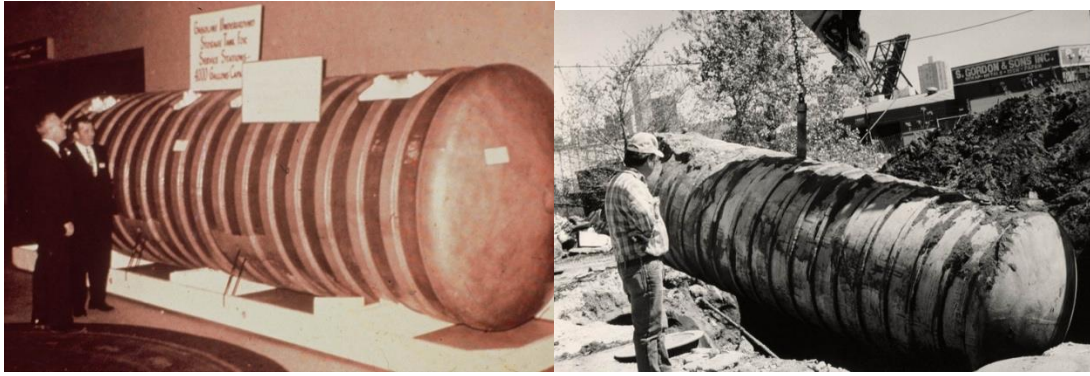
Before burial, May 15, 1963 After burial, May 11, 1988 Figure 7.1 The first generation FRP tank (courtesy of Al Dorris of Xerxes Corporation)
