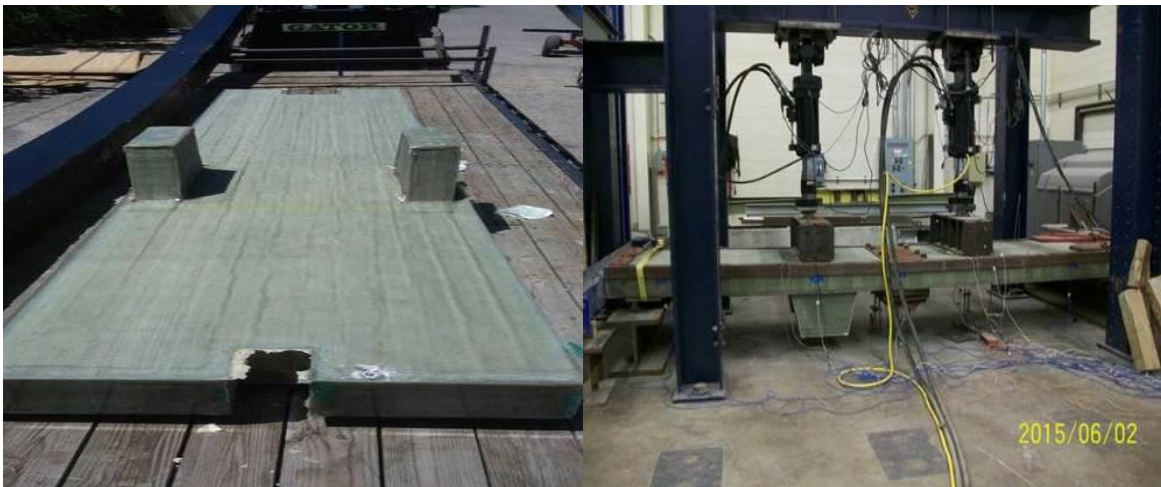
Figure 8.6 Composite Wicket Gate (Left) and Prototype Gate under Bending
