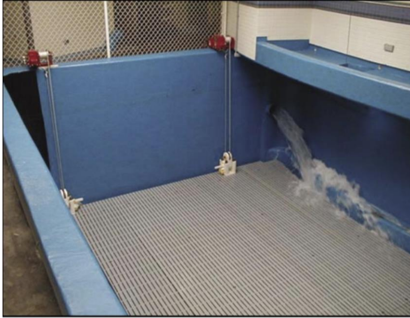
Figure 8.22 FRP lifting and lowering platform made from Strongwell products to rehabilitate the manatees
