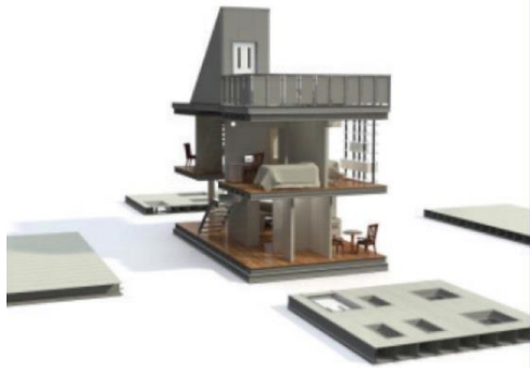
Figure 2.8 Startlink House. Startlink is a pultruded glass reinforced composite component kit which can be rapidly assembled into a wide variety of low-rise building forms without metal fastenings
