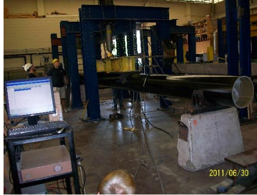
Figure 7.13 A 16" FRP Pipe Being Tested at WVU-CFC Laboratory
