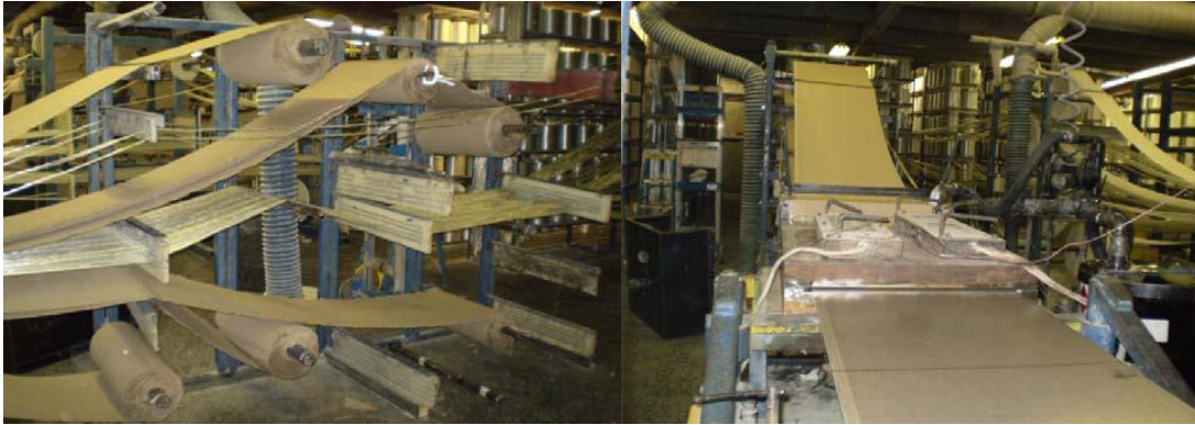
Figure 6.4 Pultrusion of Natural Fiber Reinforced Bioresin Composite Panel (Mutnuri et al, 2010)
