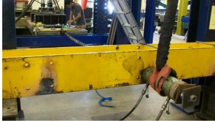
Figure 9.9 Pulling of the FRP gate with the chain attached to the top bale
