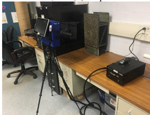
Figure 10.2 Advanced infrared testing equipment including pulsed and flashed heating and data processing computer
