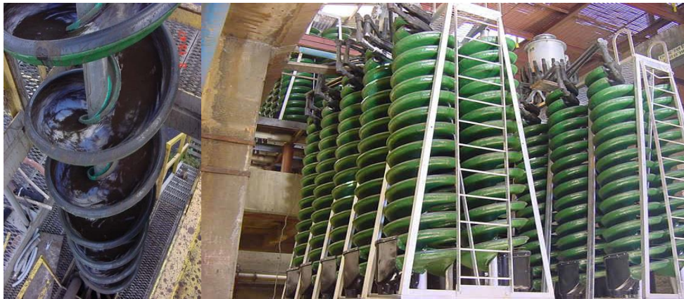
Figure 7.15 Spirals in Coal Preparation Process (courtesy of Huade)
