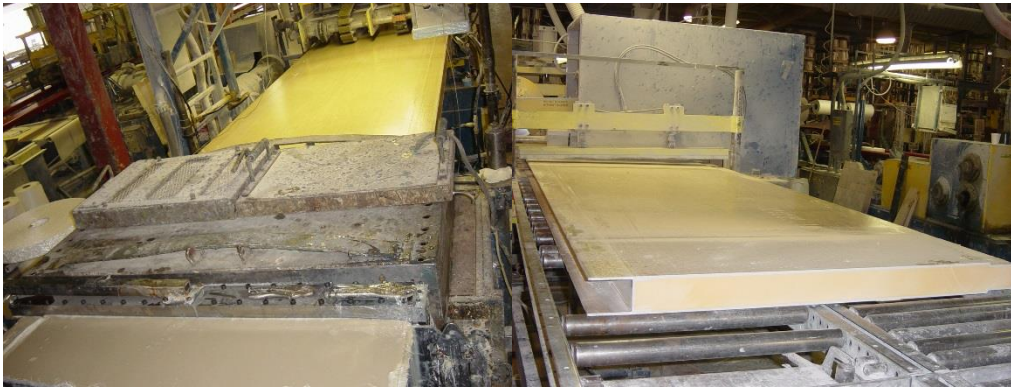
Figure 4.1 Pultrusion of 4' Wide GFRP Composite Sandwich Panels with Integral Joint Edges.
