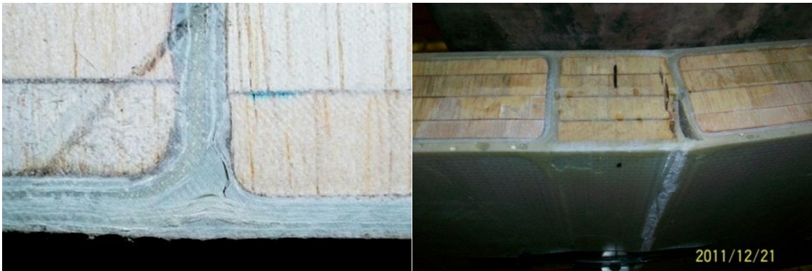
Figure 5.6 Cracking initiation and growth of a sandwich sample under 3pt bending fatigue, leading to eventual failure at the corner (WVU-CFC)
