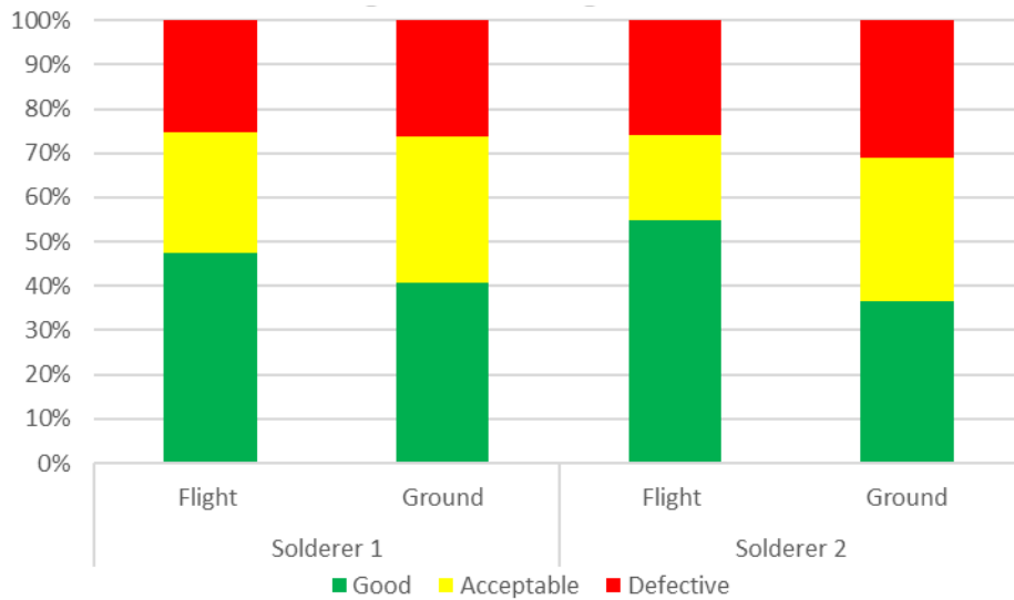
Figure 26: Quality of joints comparing flight and ground for solderers as percentage of joints they produced
