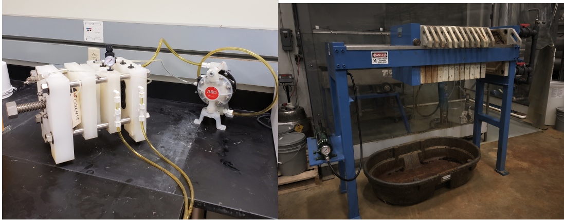
Figure 5.5 – Lab-scale 150mm filter press (left) and 420-mm filter press (right).
