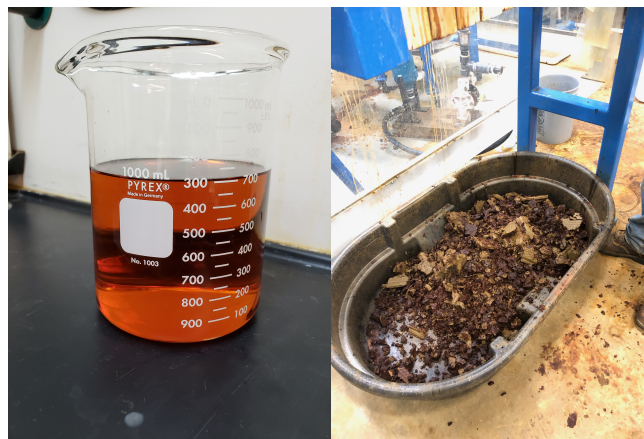
Figure 5.6 – PLS after filtration in the plate and frame filter and filter cake from clean-out of the 2 cubic-foot filter press.
