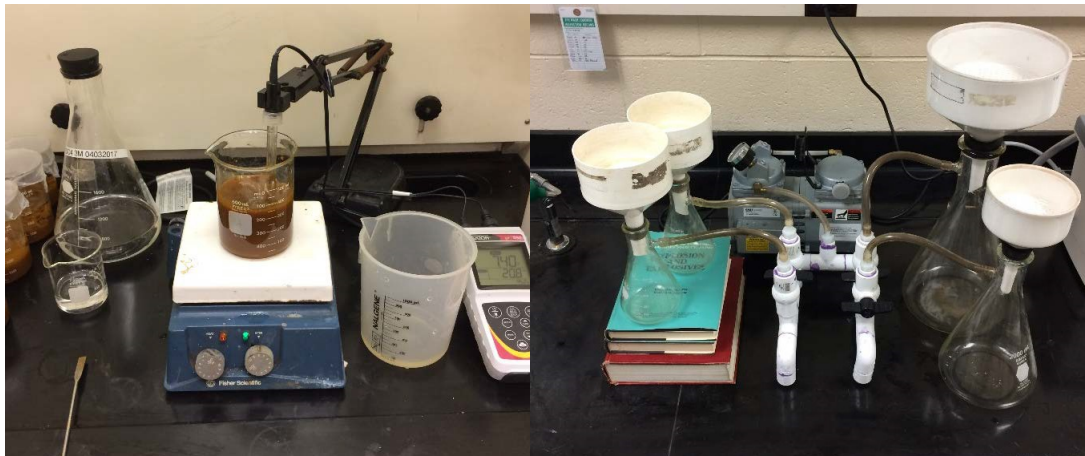
Figure 4.3 – Leaching set up and filtration manifold used for parametric testing.
