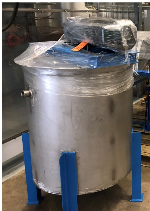
Figure 4.8 – Agitated leach tank
