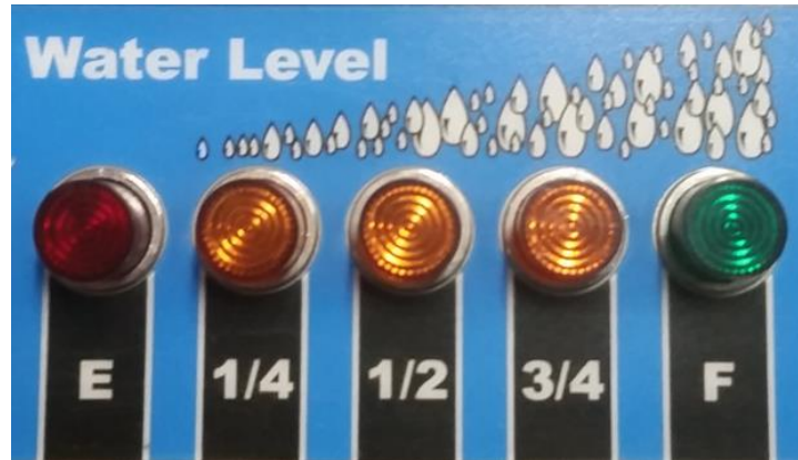
Figure 2: An LED water indicator on a Pierce pumper-tanker apparatus. [6]
