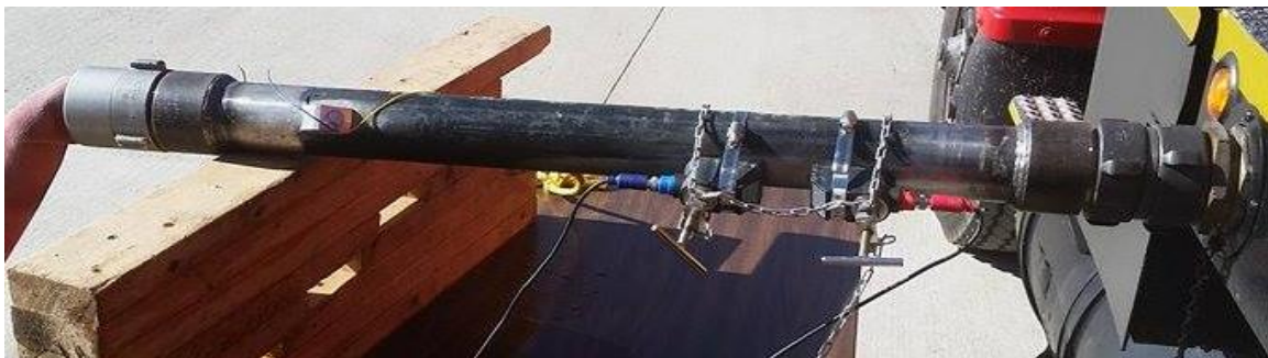
Figure 29: Image of machined adapter hooked to the inlet of a water tender
