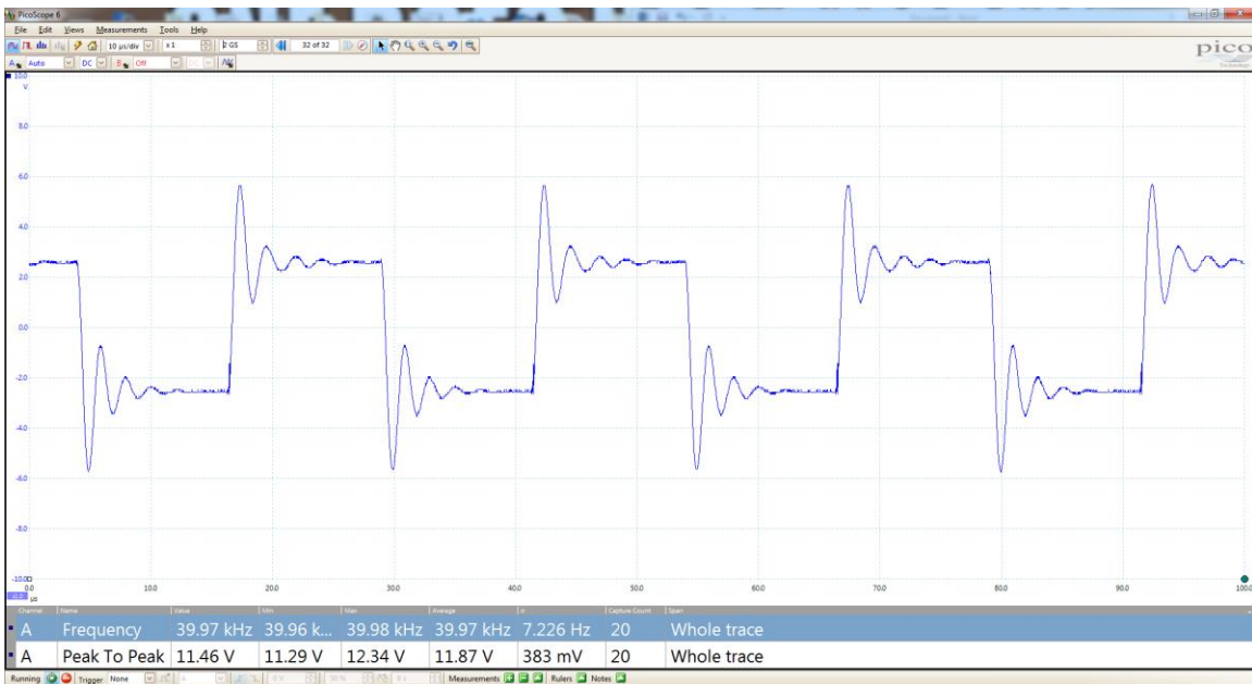
Figure 18: Test 1: 0.068 \mu F Capacitor
