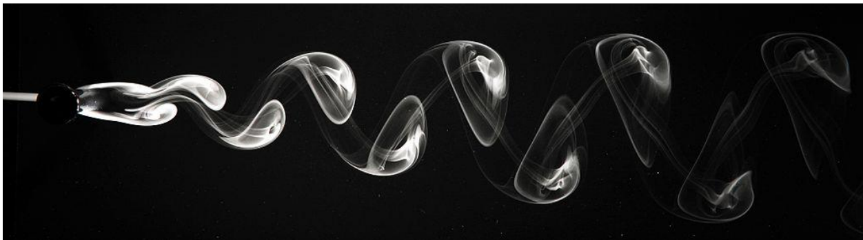
Figure 8: "Visualization of the vortex street behind a circular cylinder in air" [14]
