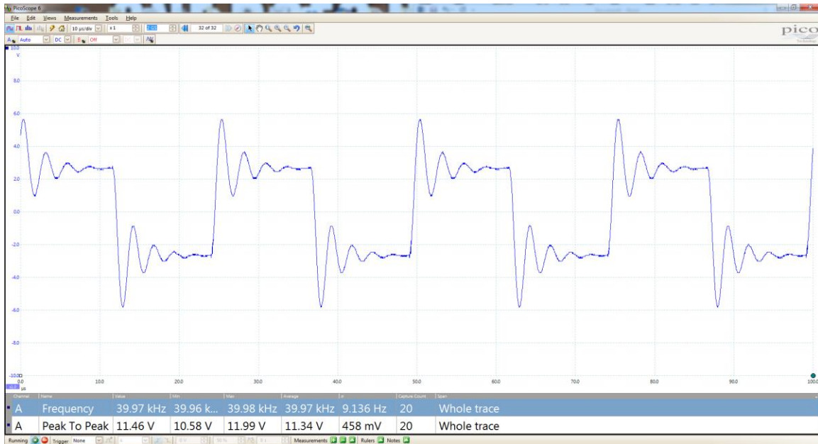
Figure 21: Test 4: 0.115 \mu F Capacitor in Parallel with 10 k \Omega Resistor
