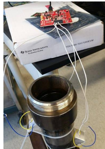
Figure 26: Example setup with milled transducer blocks affixed via cyanoacrylate
