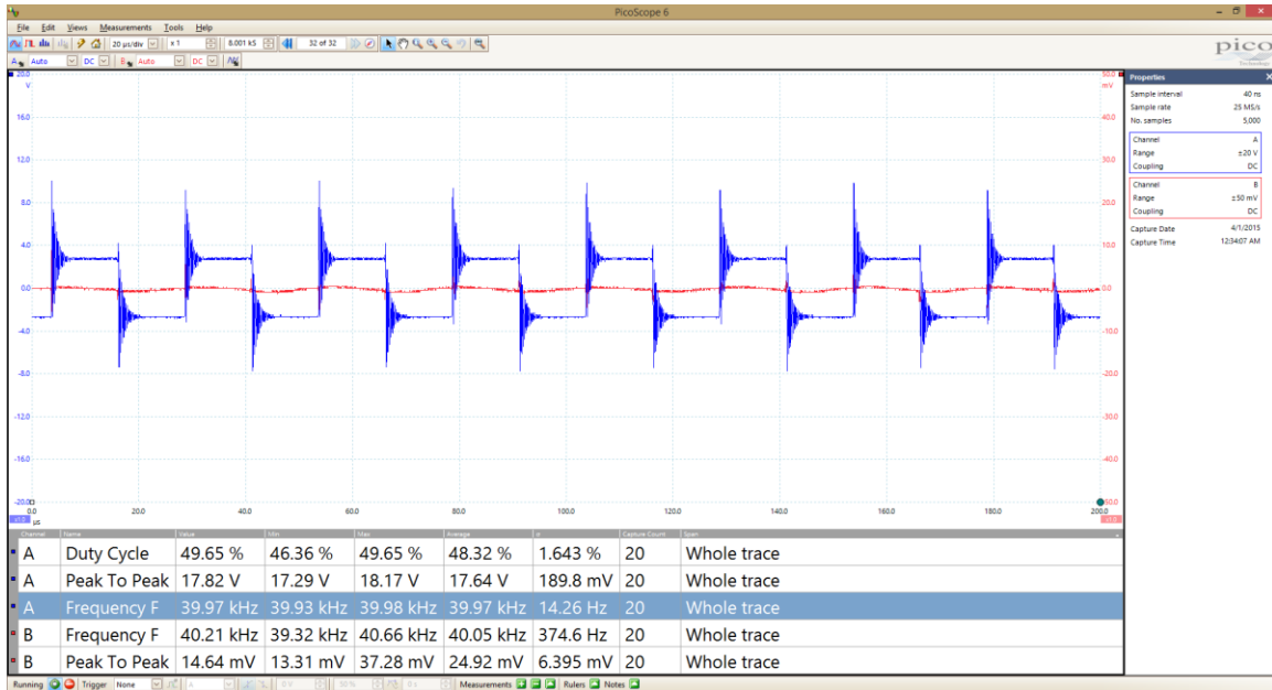
Figure 16: Empty pipe conduction test
