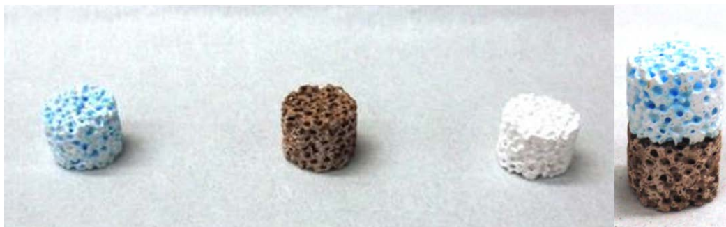
Figure 3-7 Alumina foam materials coated with reforming catalysts.
