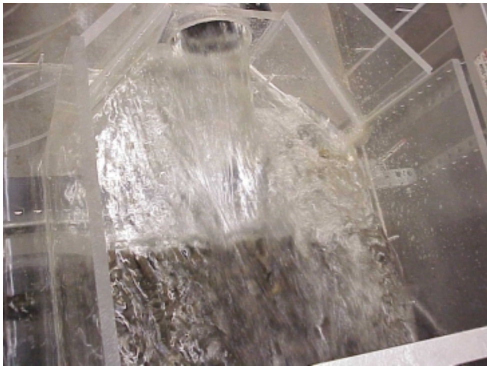
Figure 5.1 Reverse Flow in Test Channel
