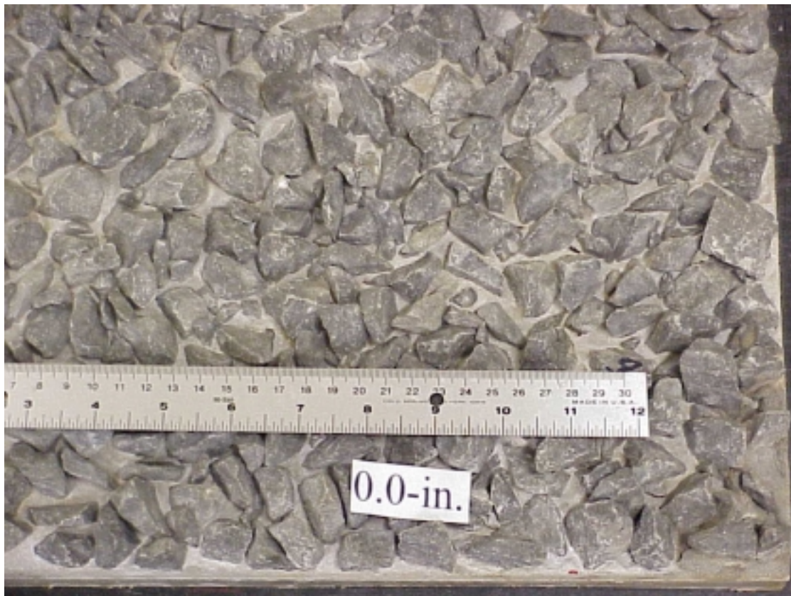
Figure 4.19 0.0-inch Equivalent Step Height
