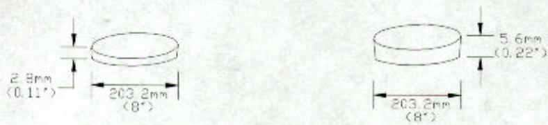
Embedded Crack Shape and Sizes (Plexiglass)
