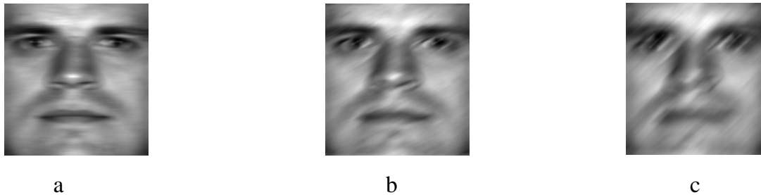
Figure 2.4: Motion blurred images at varying strengths and direction. (a) strength 15 @ 0^{\circ} angle, (b) strength 15 @ \sim 30^{\circ} angle, (c) strength 25 @ \sim 45^{\circ} angle
