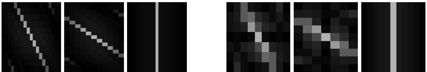
Fig 2.5: Fourier transform of filter used to simulate synthetic motion blur at varying strengths and orientation, left to right ( \sim 30^{\circ} , \sim 60^{\circ} , \sim 0^{\circ} )
