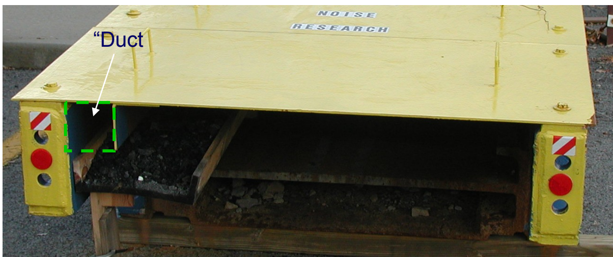
Figure 4.3 Tailpiece end of a stage loader
