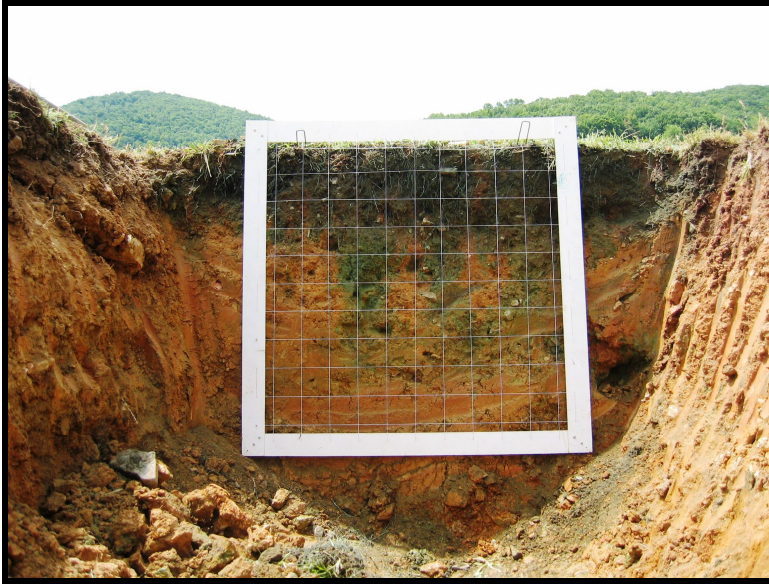
Figure 2. 4 One-meter elastic string grid framing grid for image referencing
