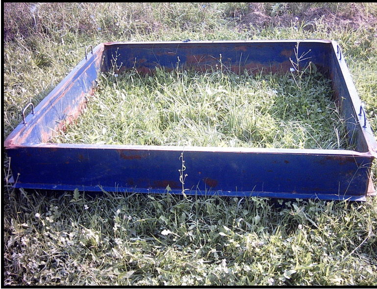
Figure 2. 3 Steel reinforced 1.3 meter by 1.3 meter dye containment apparatus used to facilitate dye ponding and infiltration
