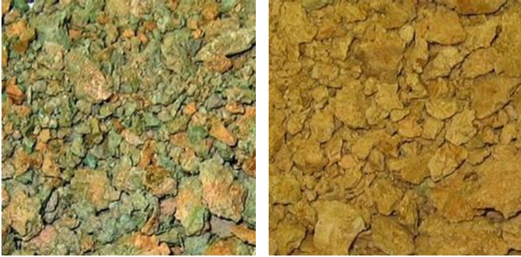
Figure 3. 3 Stained and unstained samples collected for STP analysis by Mehlich-1 extractions
