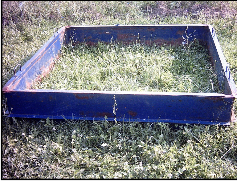
Figure 3. 2 Steel reinforced 1.3 meter by 1.3 meter dye containment apparatus used to facilitate dye ponding and infiltration
