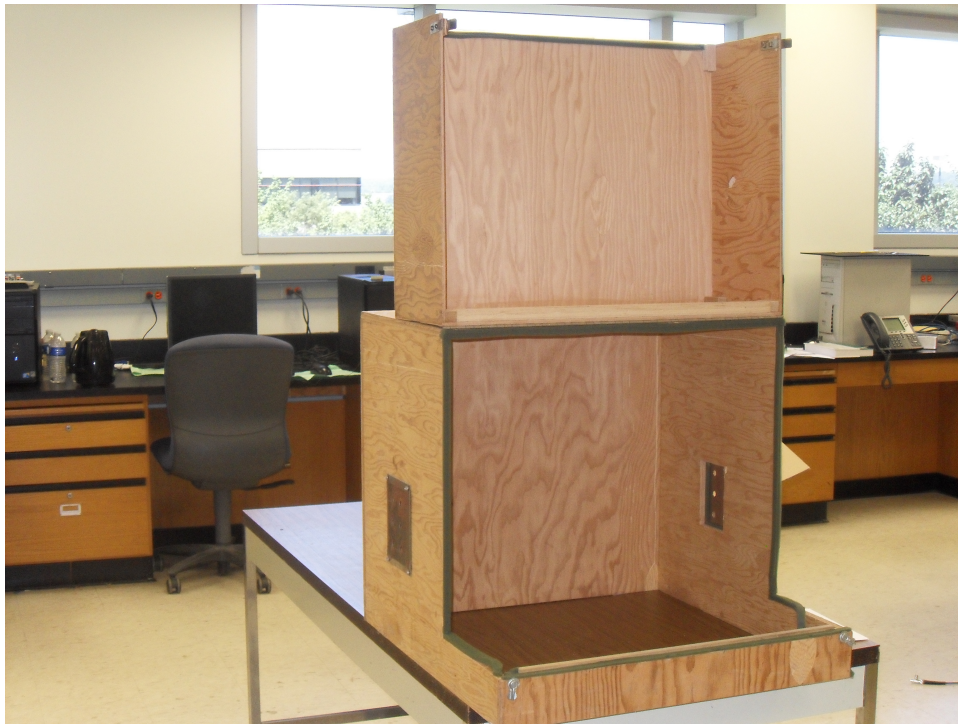
Figure 5.2: The wooden box with about 0.5 m side length that was used in the experiment.
