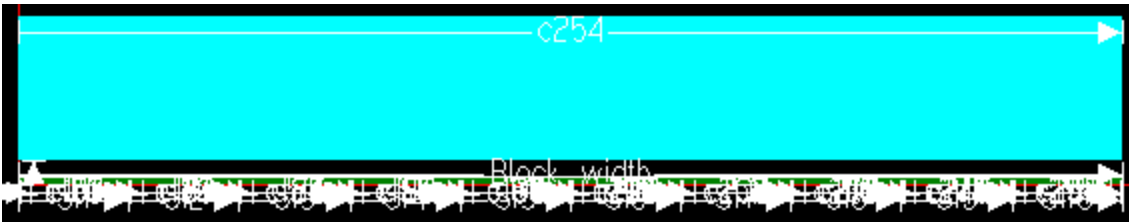
Fig 3.8 Sensor Model, consisting of 10 cells, a 1-D array with rectangular test object
