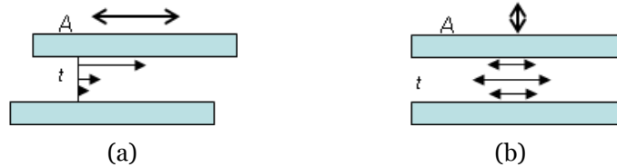
Figure 1.3.3. The damping coefficient in different movement directions.
