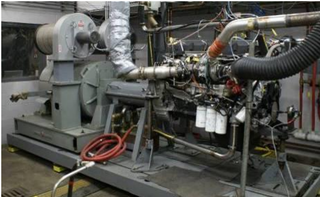
Figure 12: Test engine MY07 Volvo MD-11 [3]
