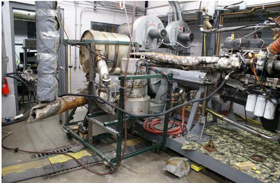
Figure 20: Connections of DPF and SCR to the engine [4]
