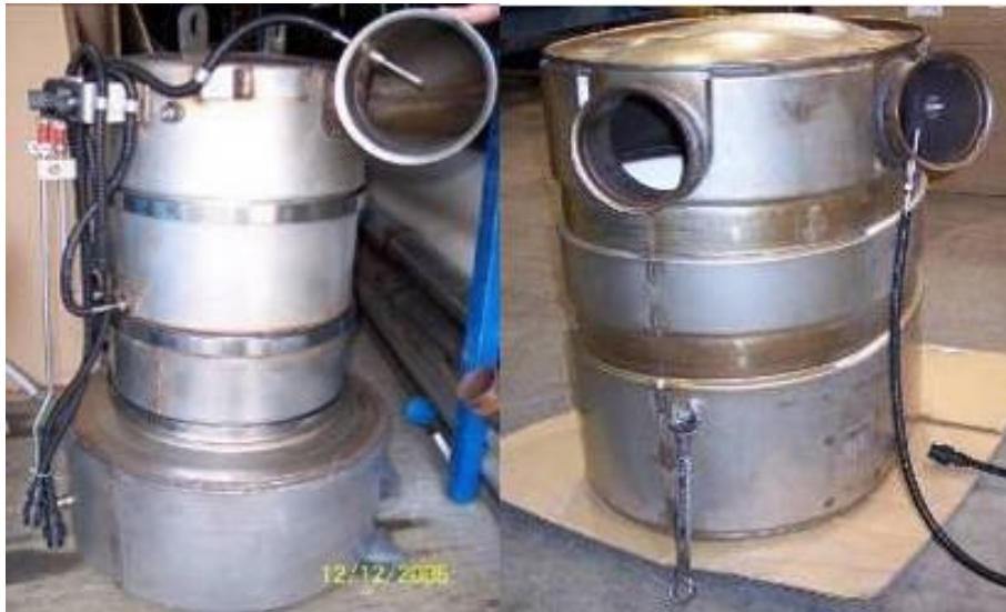
Figure 17 : Fleetgard compact DPF system and Johnson Matthey SCR system [4]
