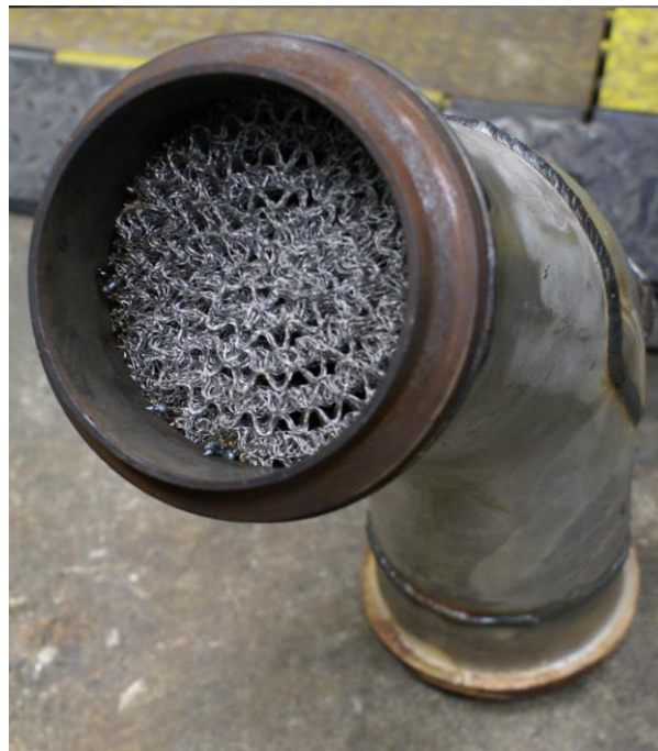
Figure 29 : Installation of wired mesh substrate in exhaust pipe
