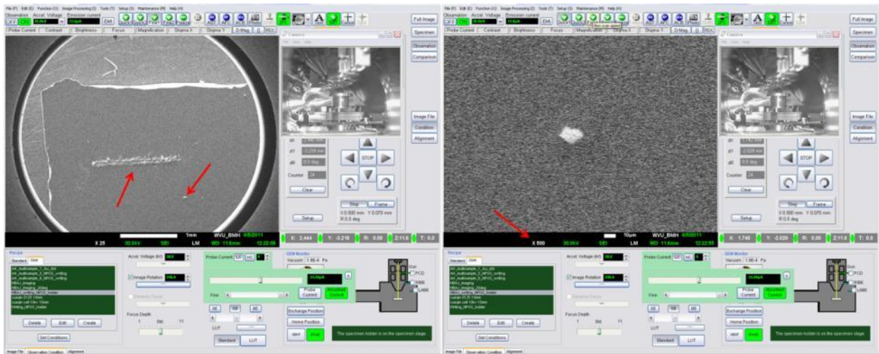
Figure B-7. The scratch area and the particle that will be used for focusing
