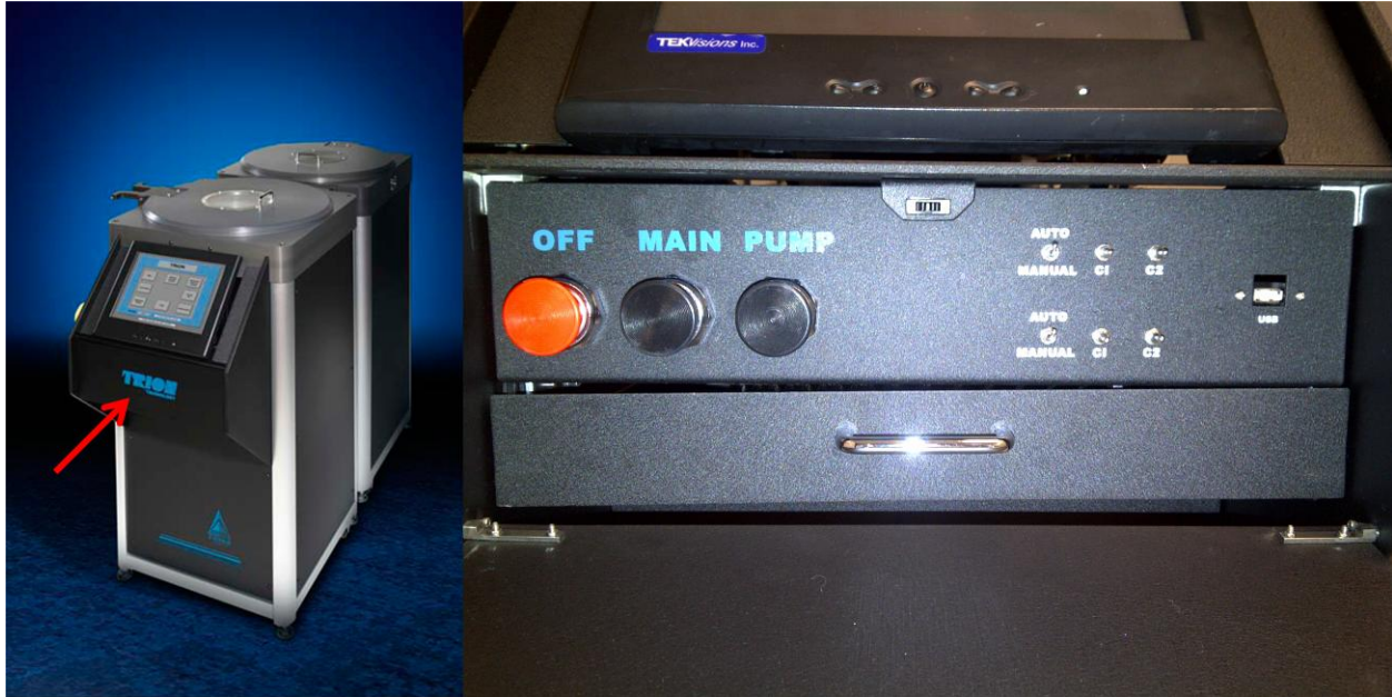
Figure D-1. The Minilock-Phantom III ICP-RIE system and the Network Tuning Controller.
