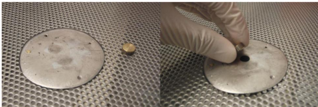
Figure C-1. Placing the SEM golden cylinder on a sputter station metal plate
