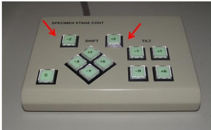
Figure B-8. Image of the Specimen Stage Controller indicating the + and - Z buttons
