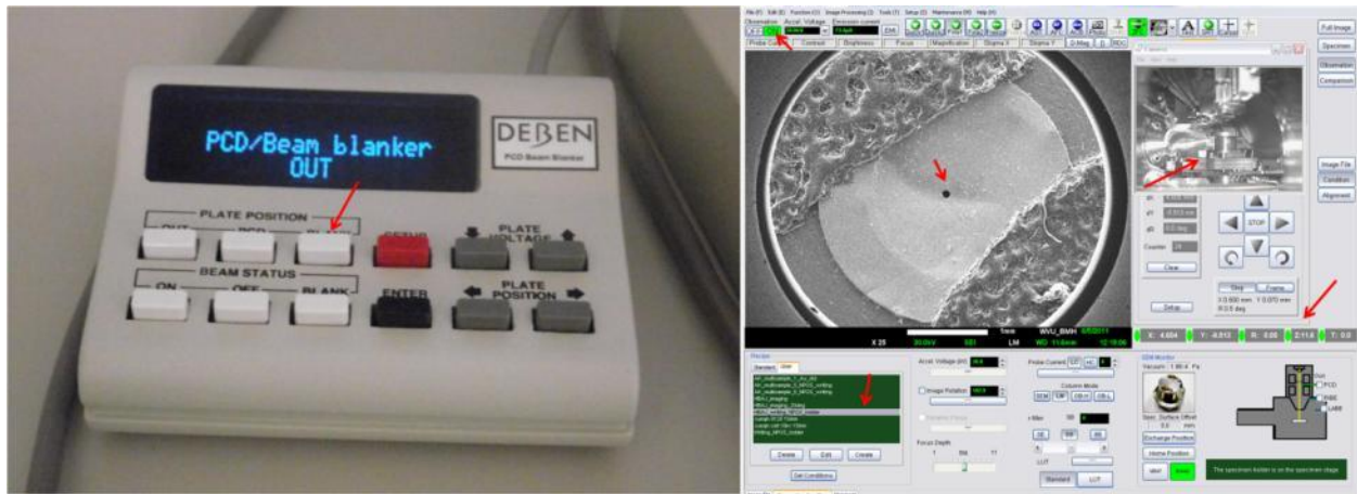
Figure B-5. Turning on the beam blaster by pushing the button indicated in the red arrow of the left image. Right image indicates the first image of the Faraday cup once the beam is turned ON in LM mode.
