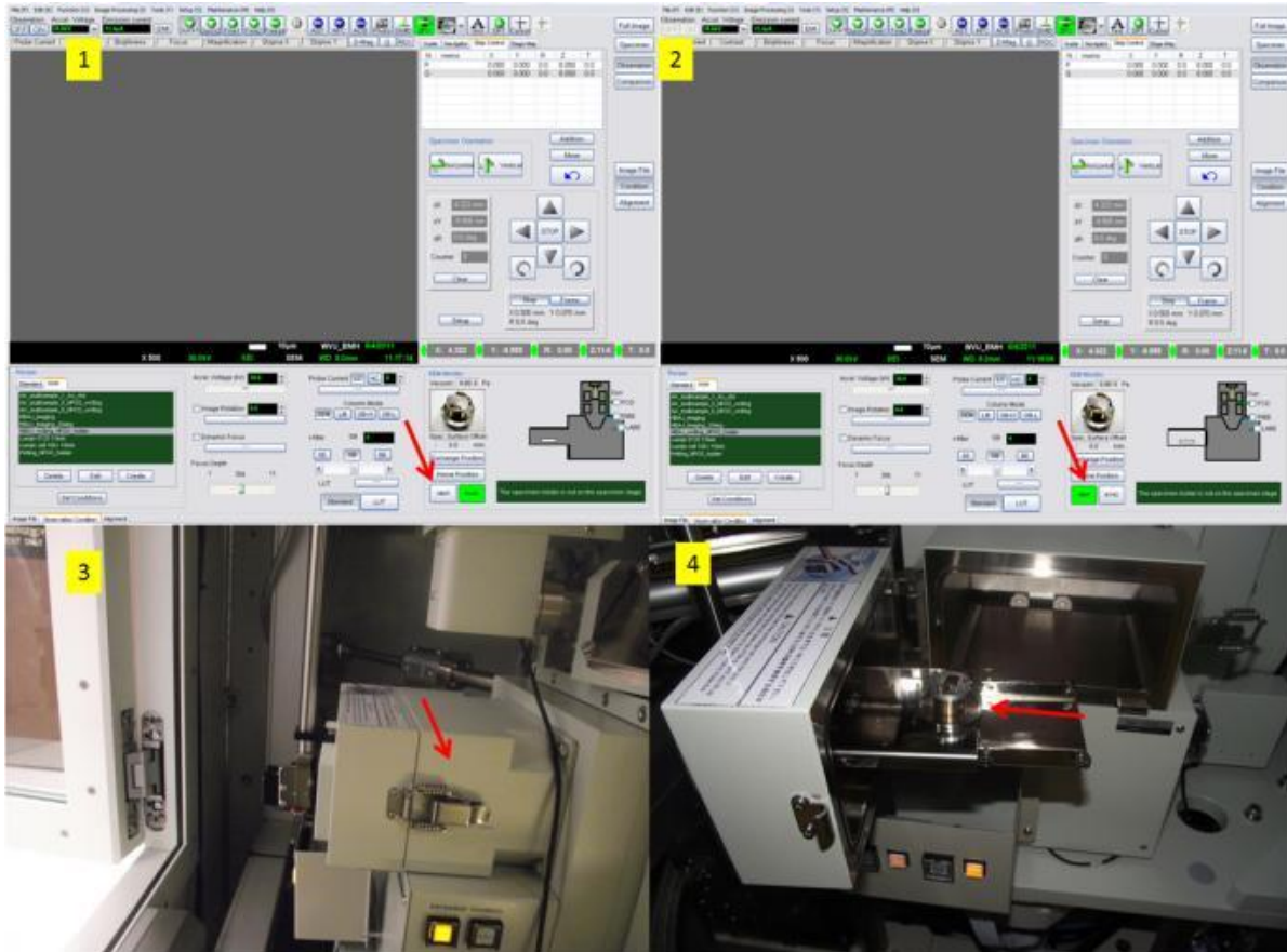
Figure B-3. Sample loading procedure. Red arrows indicate vent icon, the specimen chamber latch, and the insertion process of the sample holder.
