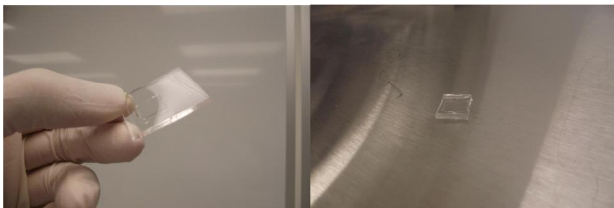
Figure C-2. Cutting the polymer sample to almost the size of the SEM golden cylinder
