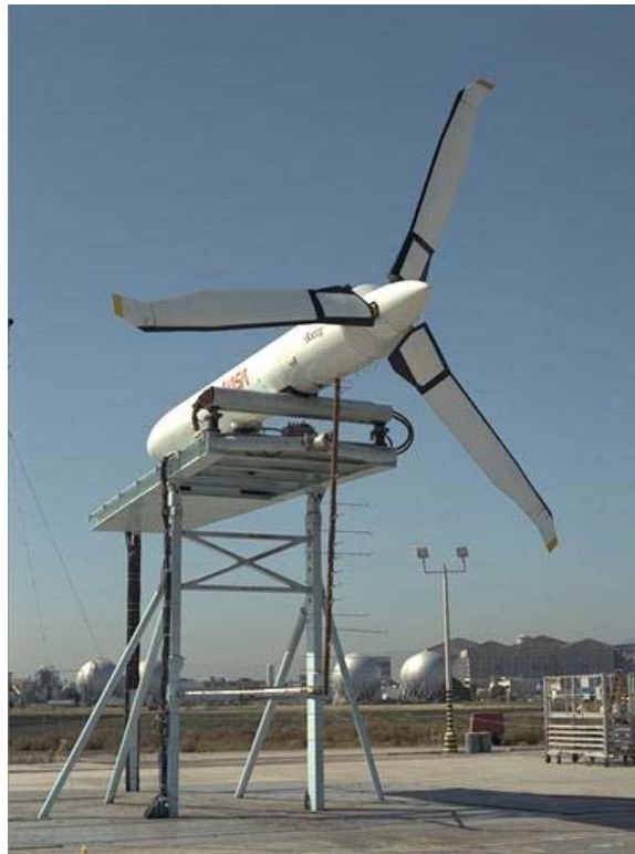
Figure 2.2 The Ames Prop Test Rig (APTR) 7
