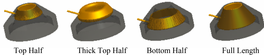
Figure 3.23: ProE Renderings of Four Cap Electrode Designs
