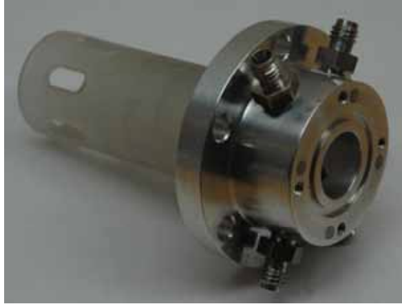
Figure 3.10: Polycarbonate and Aluminum Sump with Pipe Fittings Attached
