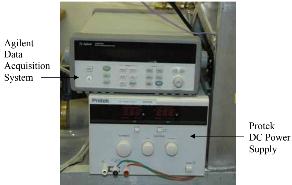
Figure 3.36: Agilent Data Acquisition System Addition and Protek DC Power Supply
