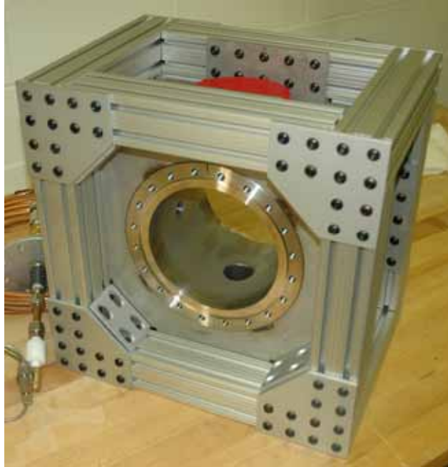
Figure 3.6: Spray Chamber with Mounting Plates and Aluminum Frame
