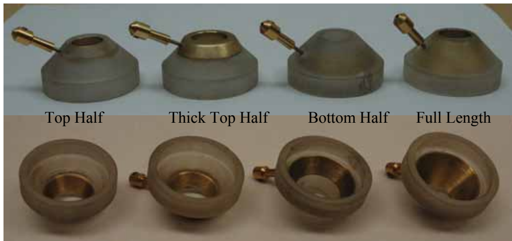
Figure 3.24: Photographs of Sides and Bottoms of Four Cap Electrode Designs with Pin Connectors
