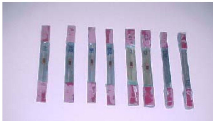
Figure 4.41 ABS Strip Tension Specimen from Belt Type (Flexible) Product and from Sheets (Last Two on the Right)
