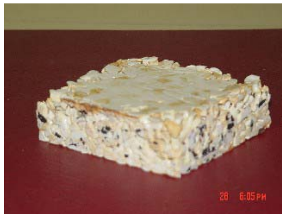
Figure 4.11 Specimen Molded With Inadequate Amount of Pellets and Solidified After Melting Under Pressure
