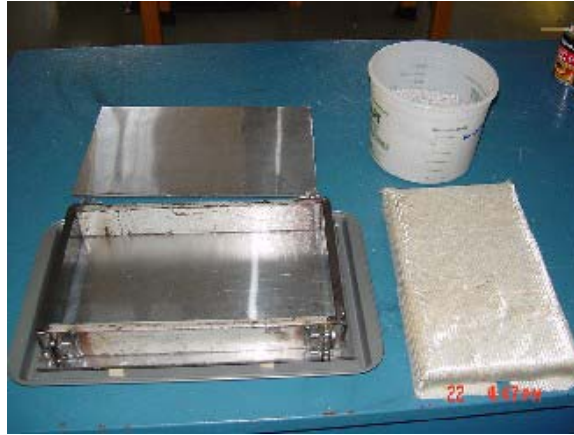
Figure 4.18 Mold Prepared for Module Manufacturing (Wrapped Core Also Shown)
