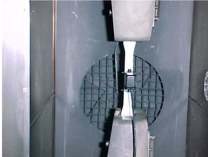
Figure 3.3 Close-up of Tension Test Set-up with Extensometer Attached
