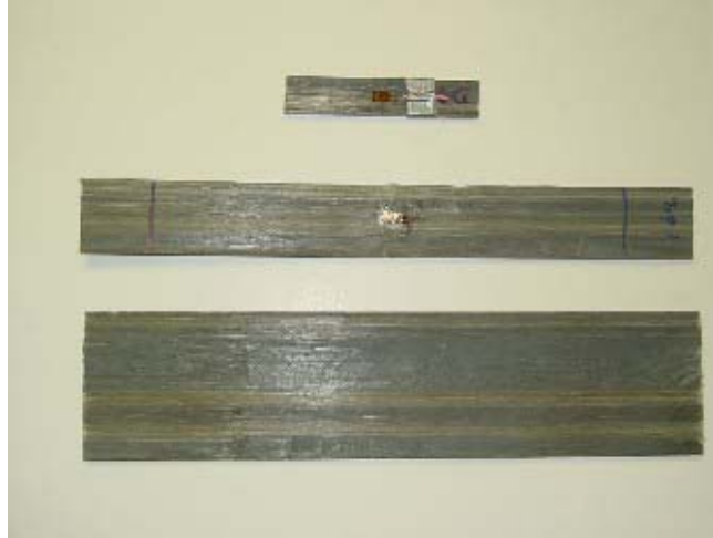
Figure 4.28 Short Plate and Long Plate Bending Specimens (With Strain Gage) Cut from Recycled ABS Sheets (Also Shown)
