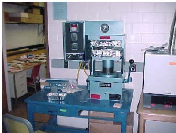
Figure 4.5 Pressure Molding Machine During Molding Process
