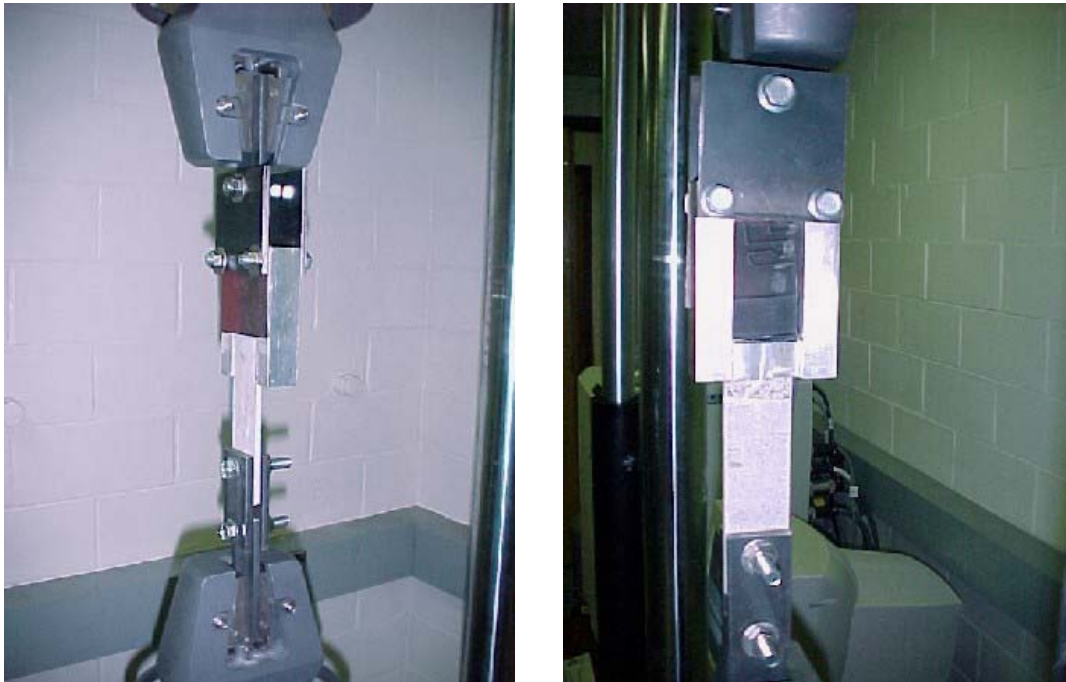
Figure 4.52 Bond Test Set-up
