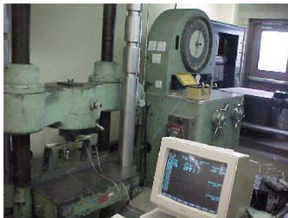
Figure 4.34 Bending Test Set-up: Universal Testing Machine and Data Acquisition System
