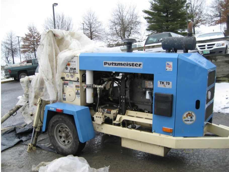
Figure 3.15: Pump used for concrete placement
