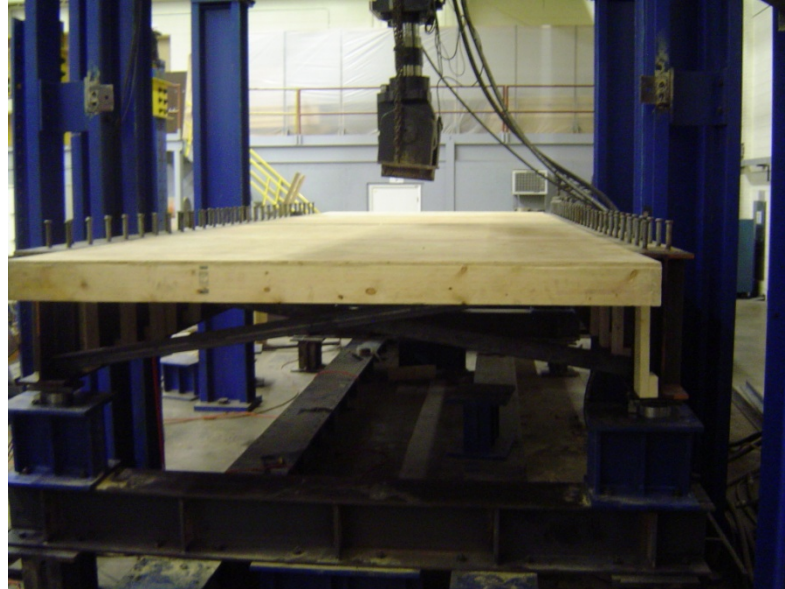
Figure 3.11: Formwork construction used for SP1, SP2, and SP3
