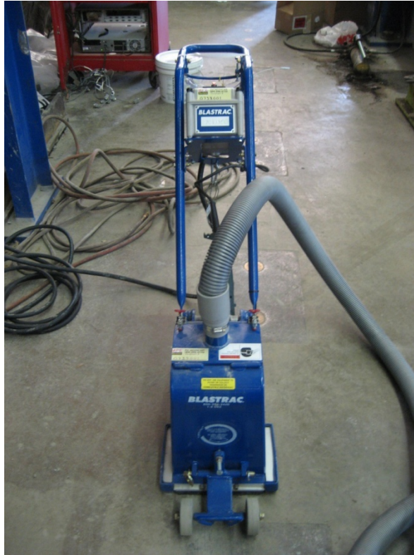
Figure 3.17: BLASTRAC used for deck scarifying
