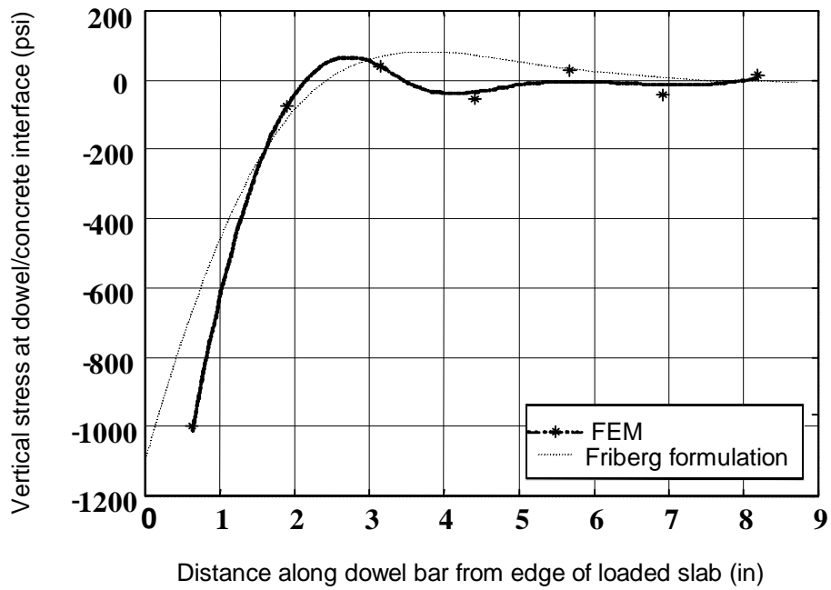
Figure 2.1 - Vertical stress distribution along dowel bar (Riad, 2001)
