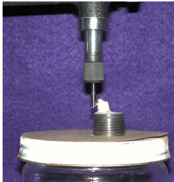
Figure 3. Use of surveyor to accurately place bracket on the tooth sample.
