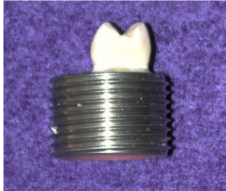
Figure 2. A sample mounted in stainless steel ring.
