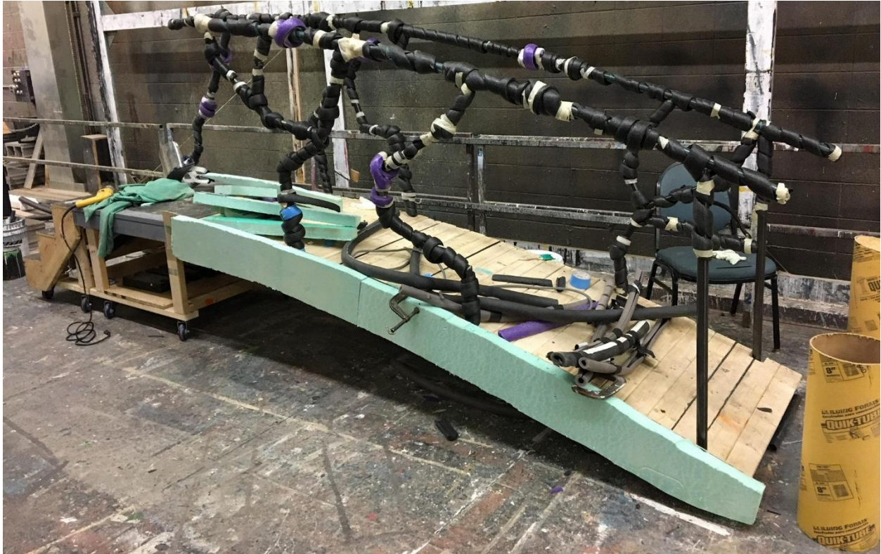
Figure 10.3 Foam Dressed on Top of Steel
