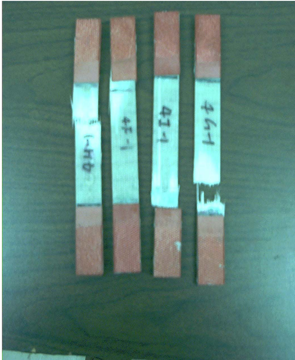
Figure 3.6 Failed Tension Test Specimens (tests 4t-7t)
