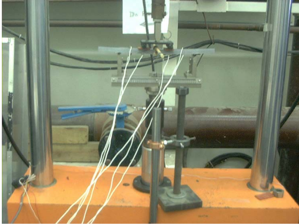
Figure 4.6 Unbent Specimen Prepared to be Loaded (B10)
