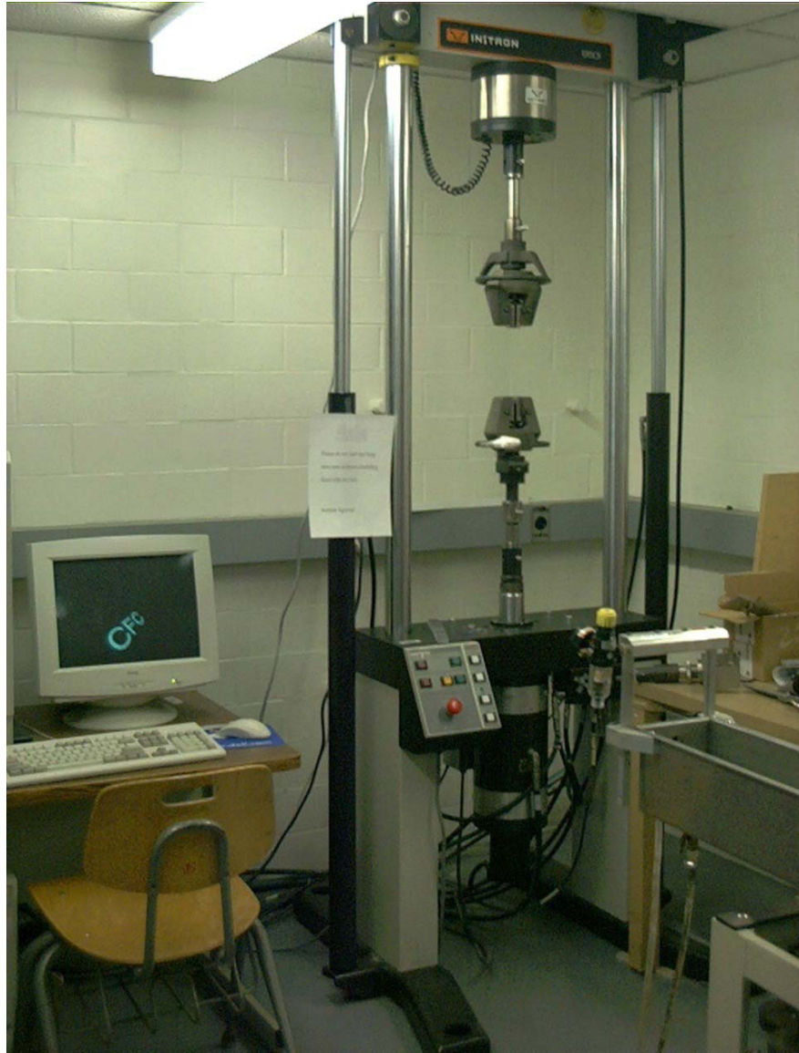
Figure 3.1 INSTRON 8501 Loading Frame, Load Cell, and Actuator
