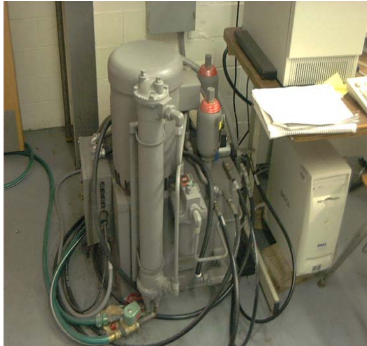
Figure 3.2 Hydraulic Power Supply
