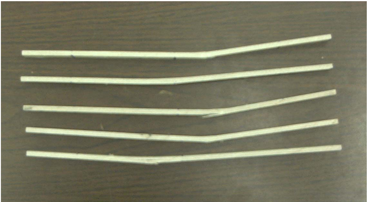
Figure 4.9 Broken Specimens, Group 2 (tests C1-C5)
