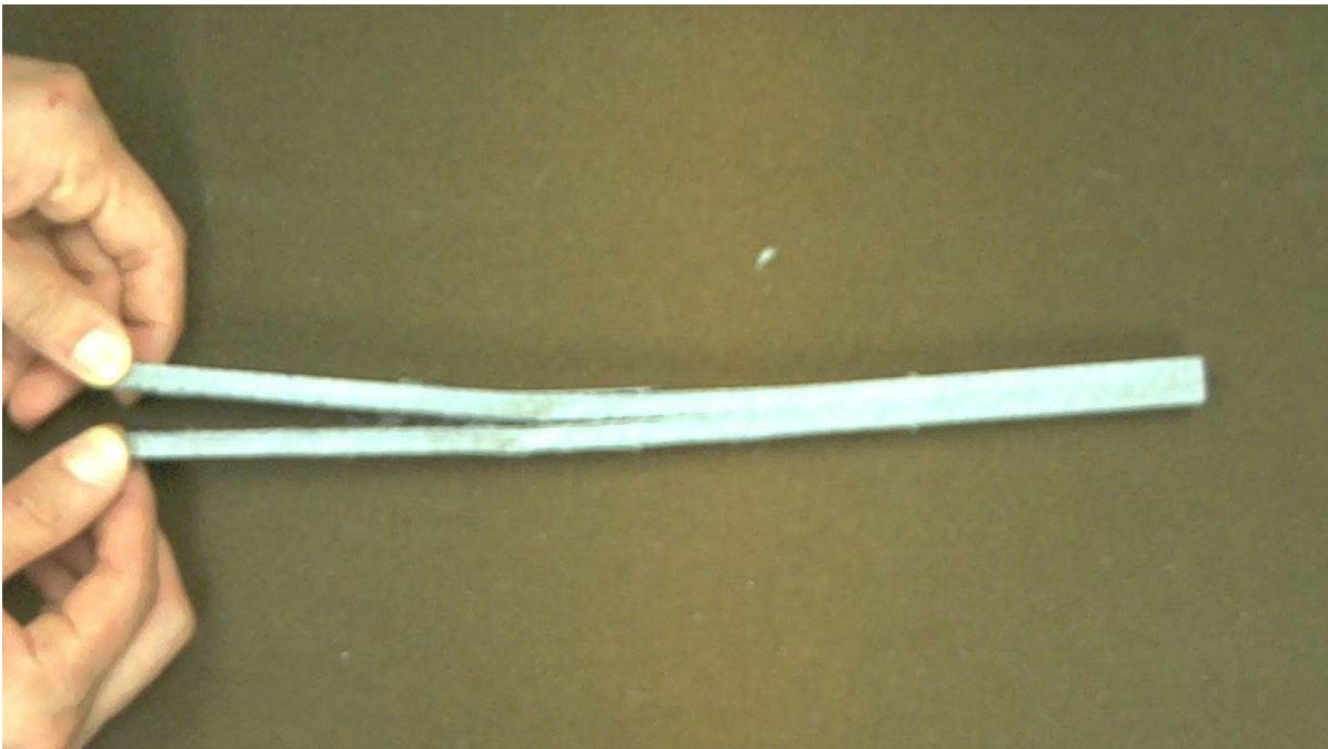
Figure 4.11 Delaminated Specimen (B9)
