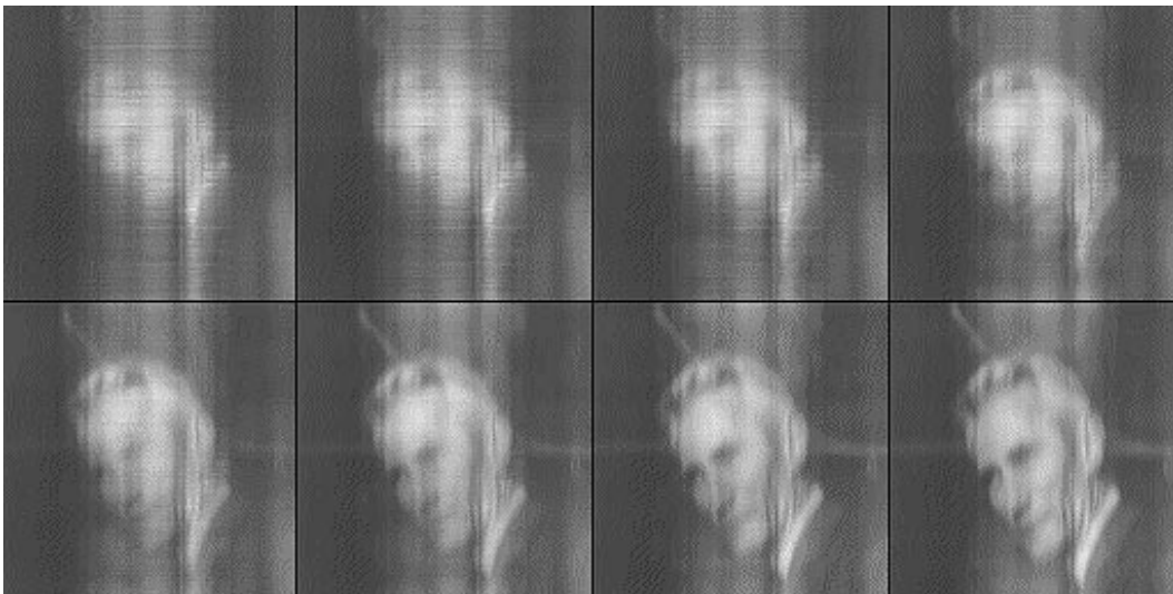
Figure 5.17: A grayscale image is applied as the input to the layer \mathbf{I} and excitation projected using the current weight matrix \mathbf{W} to the output layer \mathbf{O} is shown. Successive output images correspond to the progressively evolving \mathbf{W} weight matrix as presented above on Figure 5.16.
