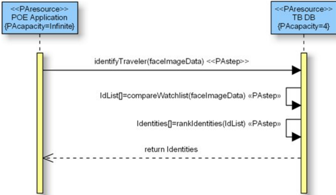
Figure 48 Sequence Diagram for the Biometric Identification Use Case
