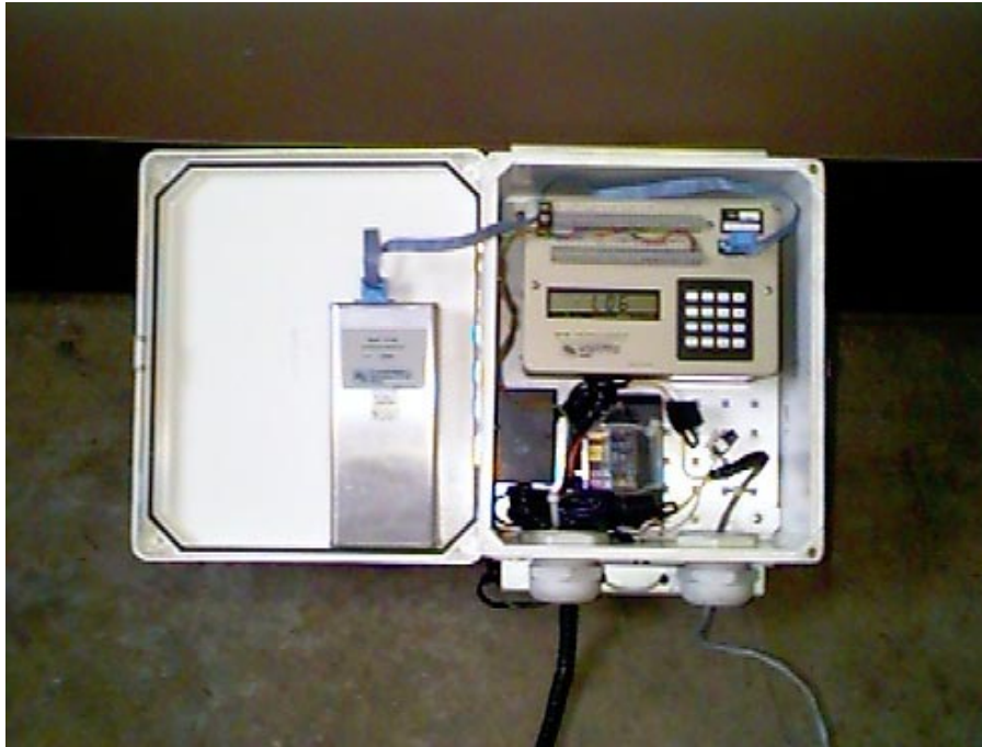
Figure 4.1.1 Campbell Scientific 21x Micrologger, used to collect speed and distance data from heavy duty vehicles.
