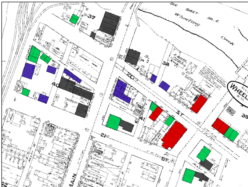
Figure 5.8 Historical GIS revealing Webster Street buildings from the 1853 city map correlated with the 1884 Sanborn map showing the quality of data sources: Level 1 models (Blue) based solely on 1853 map; Level 2 (Black) based on the correlation between 1853 and 1884 maps; Level 3 (Green) based on the 1853 and 1884 maps with local intensive survey; and Level 4 (Red) extant and/or based on photographic documentation (Steffany Wood).
