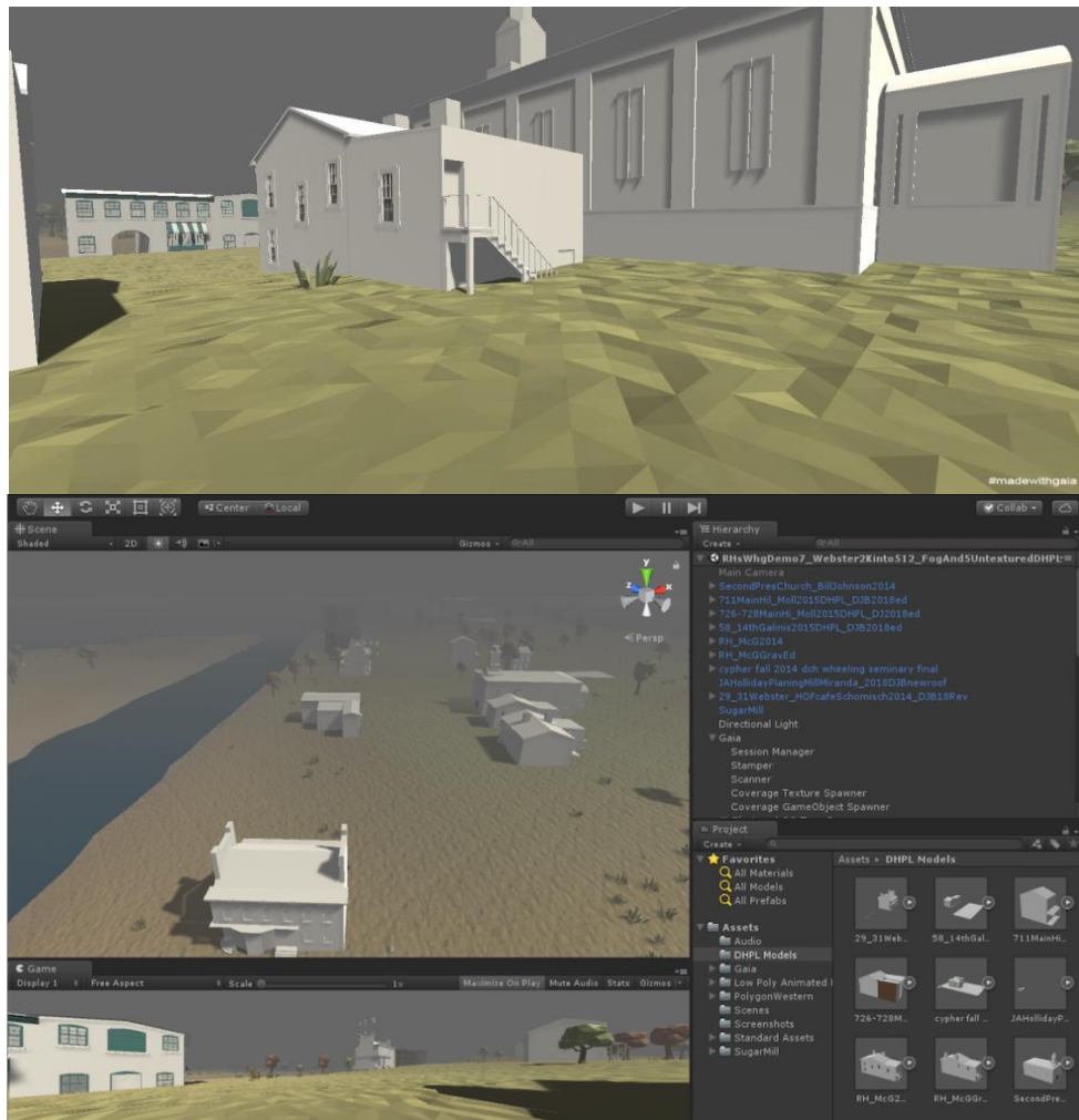
Figure 6.2 Early trial showing the height map rendered with water, vegetation, fog, and 3D building models with high polygon count. The high-polygon models functioned well in the game environment but caused the system to crash in VR.
