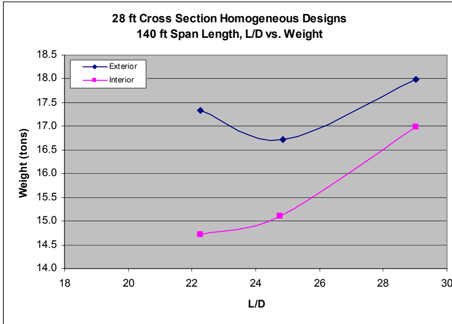
Figure 4.14 Interior vs. Exterior Girder Designs
