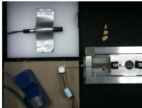
Fig. 6.10 Experimental geometry utilized during pilot DOI studies on five selected LYSO pixels. A ^{22}\text{Na} source was used to scan in depth from 1 mm to 9 mm in 1 mm steps.
