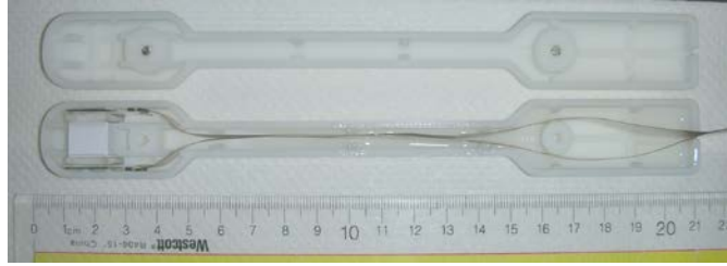
Fig. 6.7 Compact (~14 mm wide by ~20 mm high) prosate probe prototype based on the SensL dual ended readout detecotr modle. Case manufactured by Agile Technologies.
