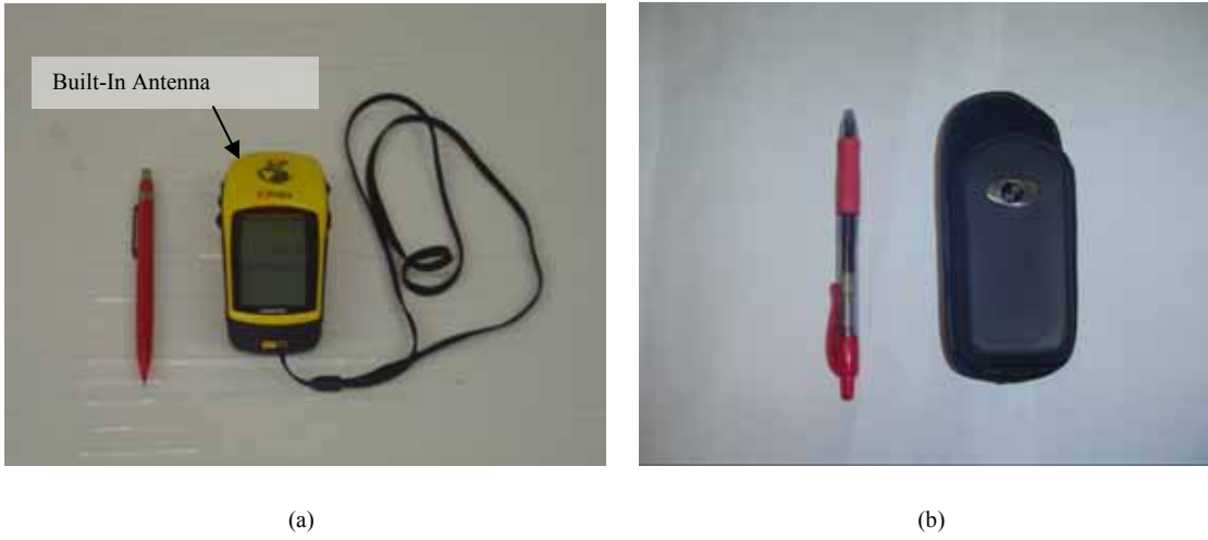
Figure 4: (a) eTrex Hand-Held GPS Device and; (b) Holster Used for This Study
