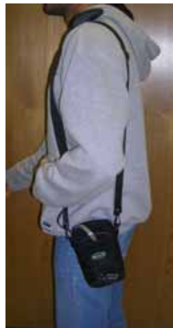
Figure 7: Wearable GPS Data-Logger Worn by a User. Note That the Antenna is Positioned on the Shoulder.
