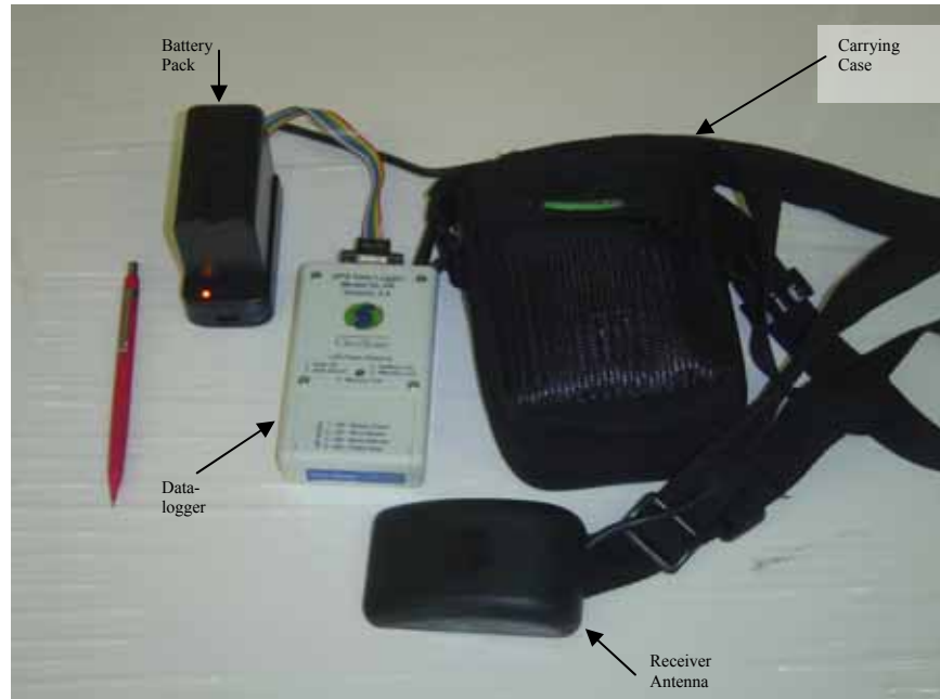
Figure 6: Components of the GPS Data Logger Used in This Study
