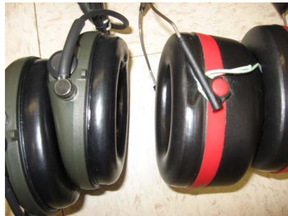
Figure 14. MSA Sordin on the left, Peltor on the right. Deeper Peltor cushion molds around anatomical features more thoroughly creating a better seal.
