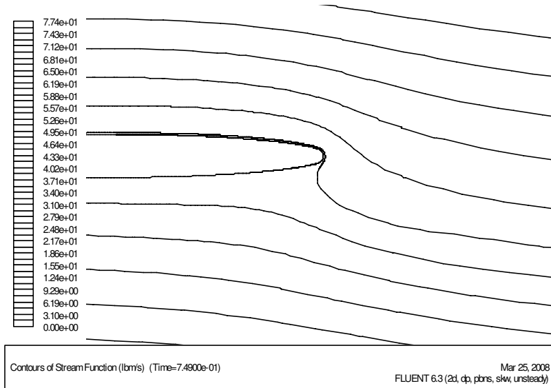
Figure I. 16: Trailing edge streamlines for LEU200TEU600
