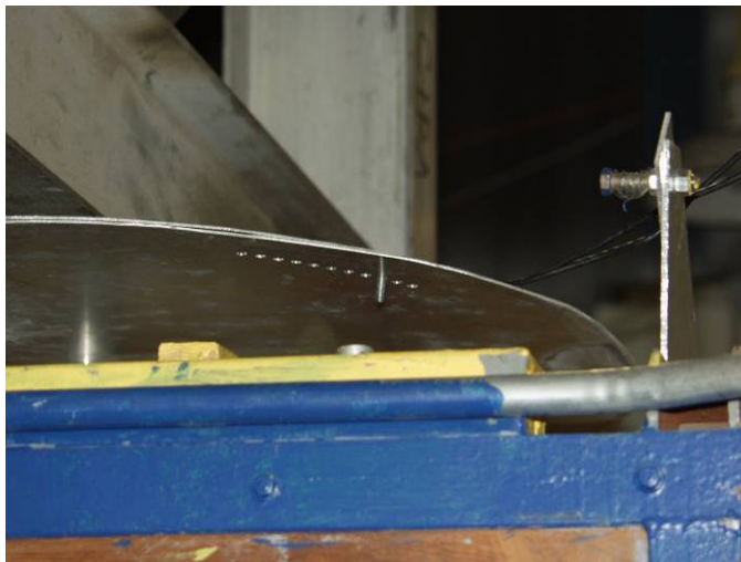
Figure 5.19: Angle of attack setting device pinned at 0 degree, indicated angle of attack
