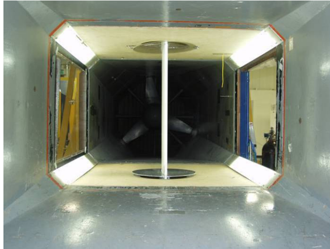
Figure 5.6: Baseline model installed in the WVU Closed Loop Wind Tunnel
