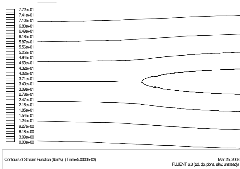
Figure I. 14: Leading edge streamlines for LEU200
