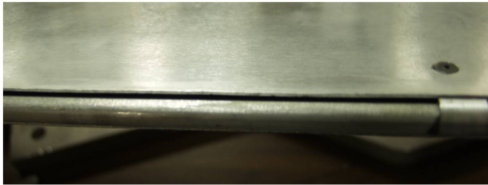
Figure 5.42: Trailing edge of the active model in the open position
