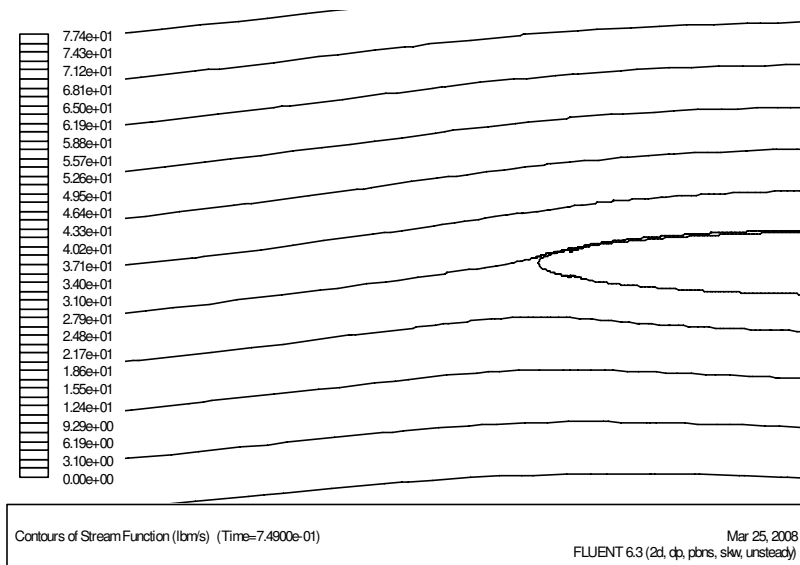
Figure I. 17: Leading edge streamlines for LEU200TEU600
