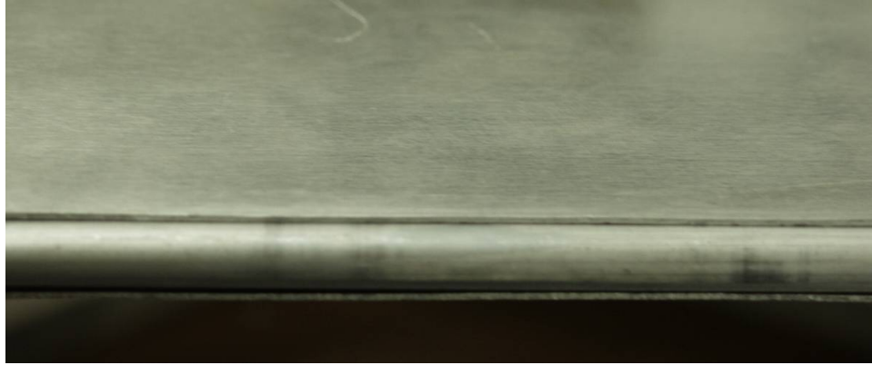
Figure 5.41: Trailing edge of the active model in the closed position
