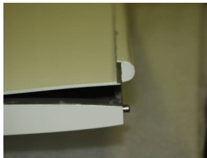
Figure 5.3: Close-up view of the assembly method for the baseline elliptic airfoil model
