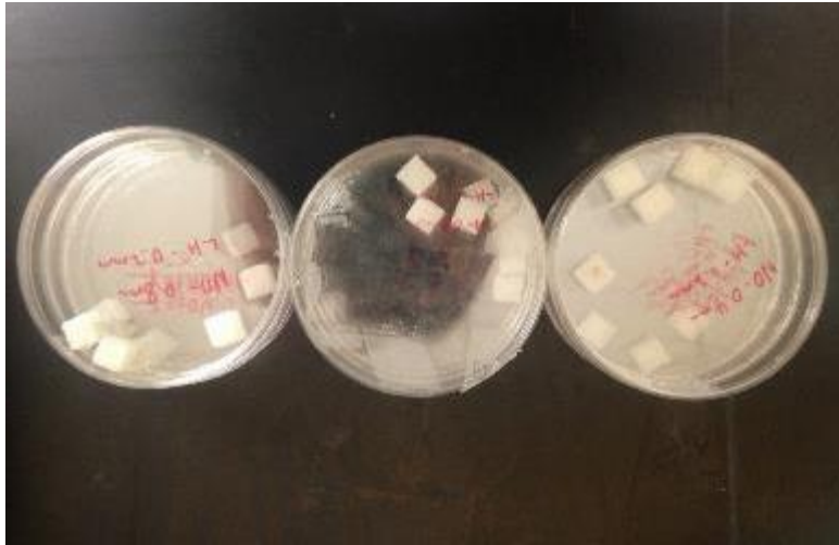
Figure 5-19 Cubic samples of Nylon 12
