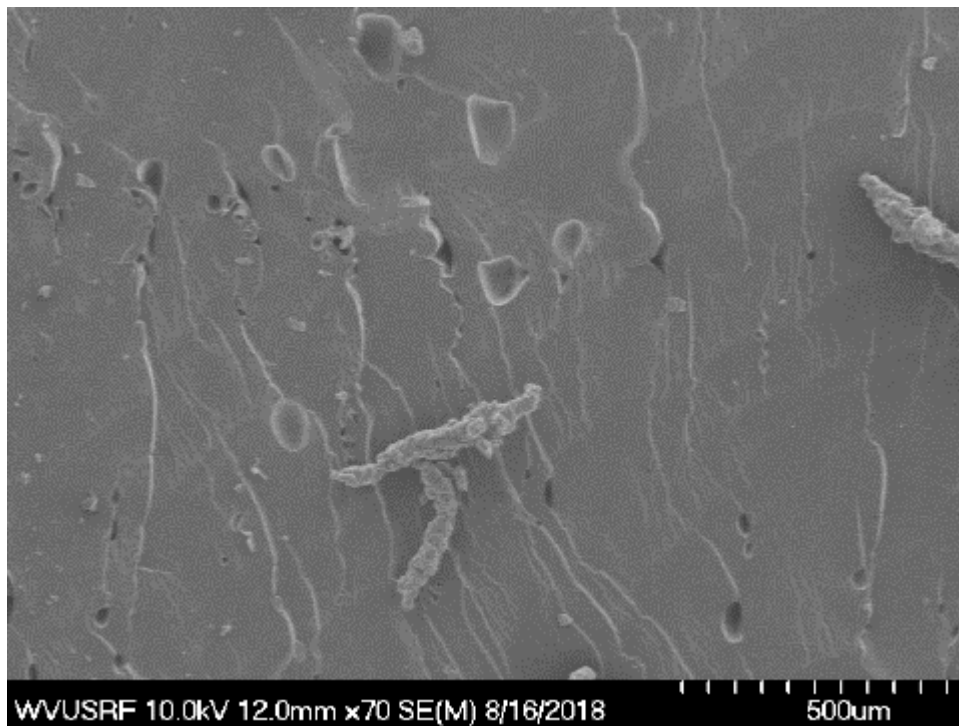
Figure 7-9 SEM image of a sample printed by 0.8mm nozzle
