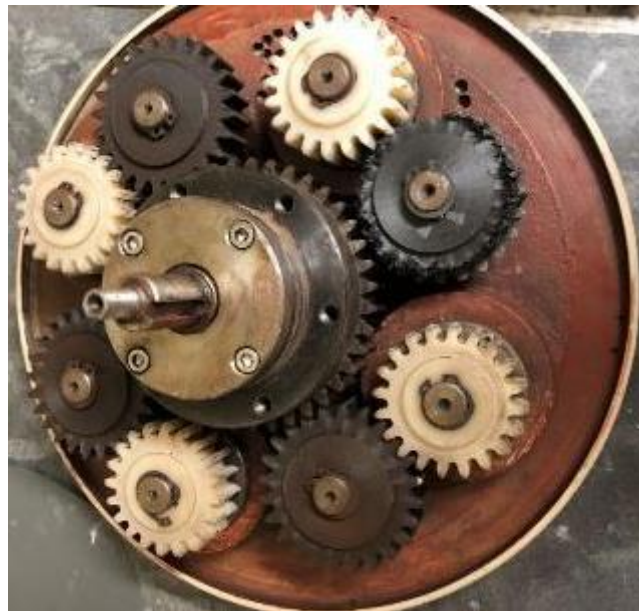
Figure 6-41 First trial of the application of CFRP gear set
