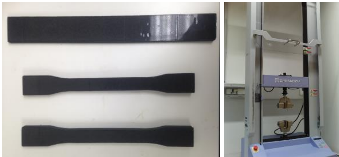
Figure 5-2 Employed specimens (a): tensile (“dog bone”, lower) and shear (rectangular, upper) and SHIMAZU tensile machine (b)
