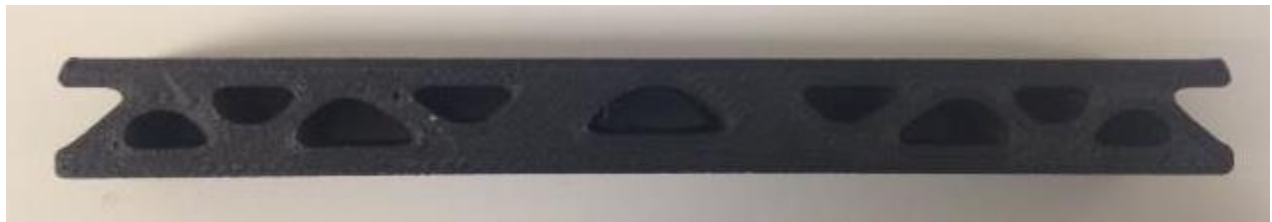
Figure 6-12 Optimized beam with carbon fiber reinforcement by FFF 3D printing
