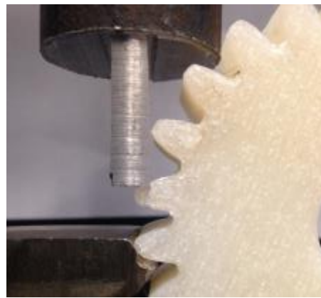
Figure 6-38 Deformed teeth of Nylon 12 spur gear
