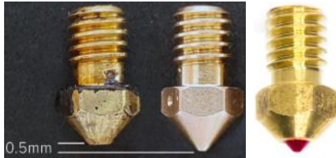
Figure 6-14 An example of nozzle damage and ruby nozzle.
