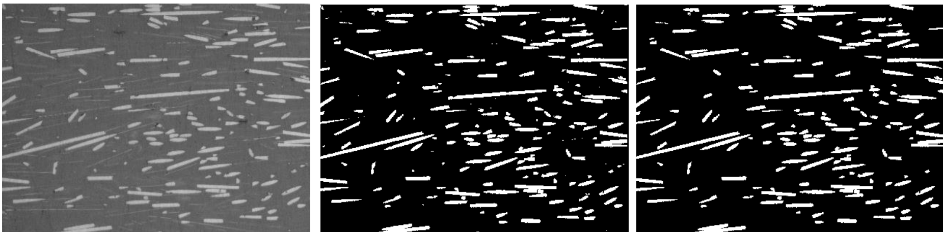
Figure 7-47 Fiber orientation computation process of a microscope image (cross-section of 90° direction, 20x)
