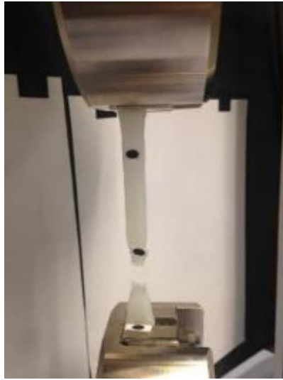
Figure 5-27 Tensile failure of a specimen printed by 0.8mm nozzle
