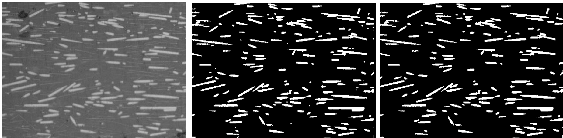
Figure 7-38 Fiber orientation computation process of a microscope image (cross-section of 90° direction, 20x)
