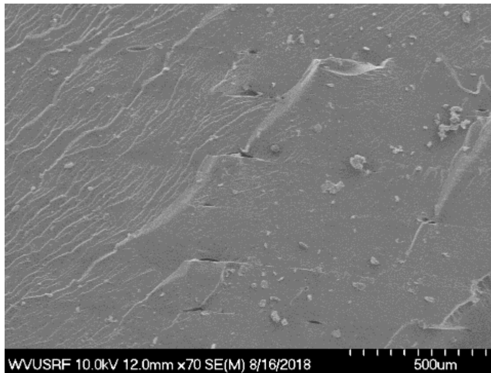
Figure 5-25 SEM image of a sample printed by 0.8 mm nozzle with 0.15mm layer height
