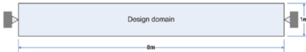
Figure 2-11 Design domain of the simply supported beam [11]
