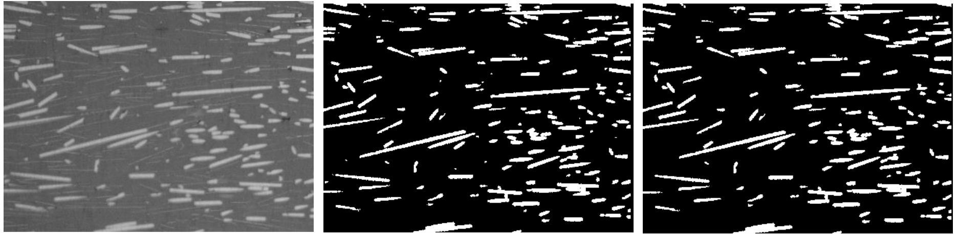
Figure 7-48 Fiber orientation computation process of a microscope image (cross-section of 90° direction, 20x)
