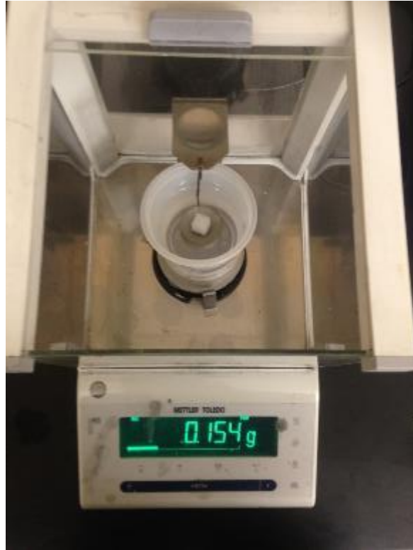
Figure 5-20 Archimedes's density measurement
