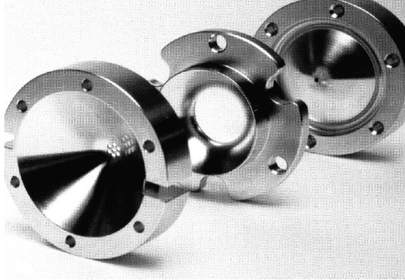
Figure 1.1. Exhibition of three electrodes: one ring electrode being sandwiched by two end-cap electrodes. Reproduced from reference [1] with permission.
